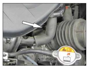
5. Loosen the hose clamp securing intake tube to the throttle body.
