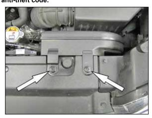
2. Loosen and remove the plastic screws securing the fresh air scoop.
