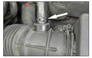
4. Release the spring clamp securing the crank case vent hose to the intake tube and then disconnect the crank case vent hose.
