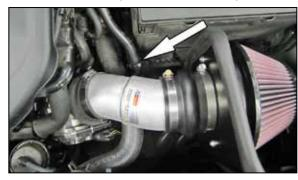
19. Install the crank case vent hose onto the 90° fitting and secure with the factory spring clamp.
