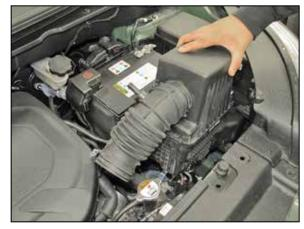
7. Lift up and remove the air box and intake tube from the vehicle.
