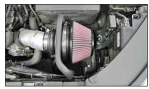
18. Install the K&N® air filter onto the filter adapter and secure with the provided hose clamp.
