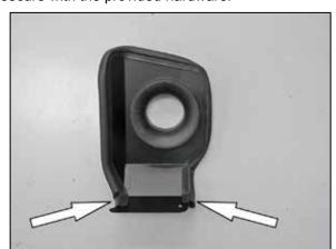
10. Install the provided edge trim around the heat shield as shown.
