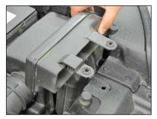
3. Pull up and remove the fresh air scoop from the vehicle.
