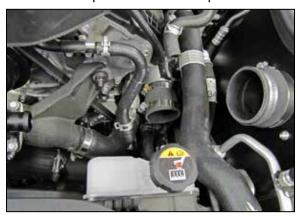
14. Install coupling hose (08638) onto the turbo inlet and secure with the provided hose clamp.
