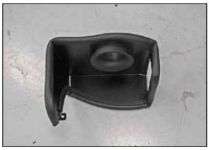
19. Install the edge trim onto the passenger side heat shield as shown.
