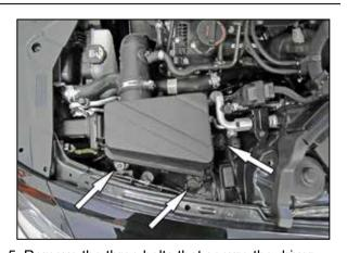
side air filter housing to the inner fender, loosen the hose clamp that secures the intake tube to the air filter housing and disconnect the tube. Remove the driver side air filter housing from the vehicle.
