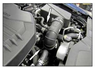
vent lines attached to the driver's side intake tube and then disconnect the vent lines from the intake
