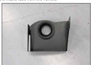
10. Install one of the two provided filter adapters into the driver side heat shield (073252) as shown and secure the adapter with the provided hardware.
