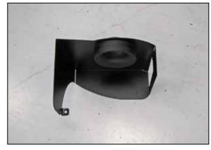
18. Install the remaining filter adapter into the passenger side heat shield (073253) as shown and secure the adapter with the provided hardware.
