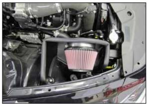
21. Install the passenger side heat shield assembly into the vehicle so the fresh air intake inserts into the opening of the heat shield and then secure the heat shield with the provided hardware.
