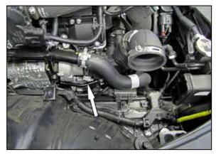
9. Loosen the hose clamp that secures the intake tube to the passenger side turbo and then remove the intake tube from the vehicle.
