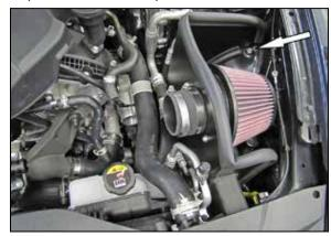
13. Install the driver side heat shield assembly into the vehicle so the fresh air intake inserts into the opening of the heat shield and then secure the heat shield with the provided hardware. Install the coupling hose (084036) onto the filter adapter and secure with the provided hose clamp.
