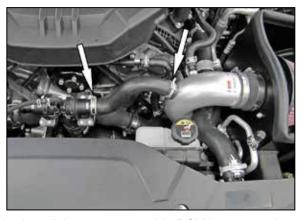
17. Install the passenger side BOV hose onto the driver side intake tube and BOV valve, secure with the factory spring clamps. Connect the vent lines to the fittings installed into the K&N® intake tube.
