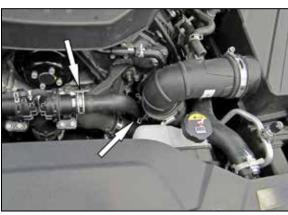
4. Release the spring clamps that secure the driver side BOV hose to the BOV and intake tube, then remove the driver side BOV hose.
