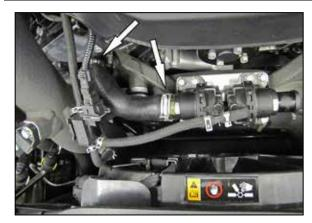
7. Release the spring clamps that secure the passenger side BOV hose to the BOV and intake tube, then remove the driver side BOV hose.
