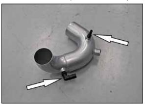
15. Install the NPT vent fittings into the driver side  $K\&N^{\otimes}$  intake (27677) as shown.
