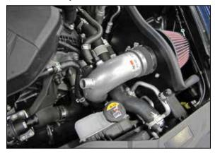
16. Install the driver side intake tube (27677) into the coupler at the turbo and then into the coupler at the filter adapter, adjust the tube and heat shield assembly for best fit and then secure with the provided hose clamps.
