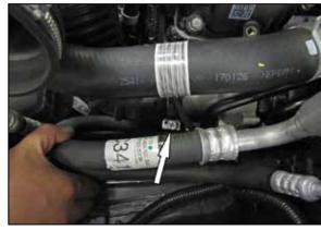
6. Loosen the hose clamp that secures the intake tube to the driver side turbo and then remove the intake tube from the vehicle.
