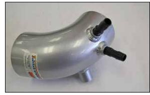
13. Install the two provided NPT fittings into the intake tube as shown.
