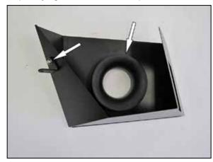
9. Install the provided heat shield mounting bracket and filter adapter onto the heat shield and secure with the provided hardware.
