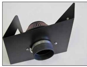
11. Install the provided coupler (08698) onto the filter adapter and secure with the provided hose clamp.
