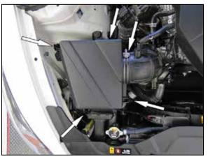
4. Release the four-upper air filter housing retaining clips and loosen the hose clamp that secures the housing to the intake tube. Remove the upper housing from the vehicle. 5. Remove the three bolts that secure the factory lower air filter housing to the inner fender and then remove the housing from the vehicle. **NOTE: K&N Engineering, Inc., recommends that customers do not discard factory air intake.**
