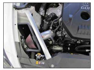
16. Reinstall the chassis brace and secure with the factory hardware.
