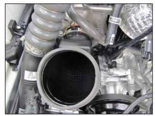
8. Reinstall the turbo inlet tube clocked slightly left from the factory location (The locating tab will be positioned just left on the turbo from factory) and secure with the provided hose clamp. Do not completely tighten the hose clamp at this time.
