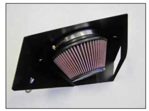
10. Install the air filter onto the heat shield and
