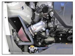
14. Install the heat shield assembly and intake tube as a unit into the vehicle. Secure the heat shield using the provided hardware. Adjust the intake tube for best fit and secure with the provided hose clamps.
