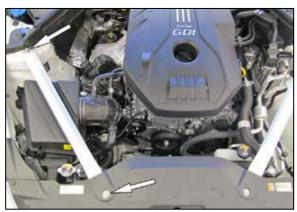
2. Remove the two bolts that secure the passenger side chassis brace and then remove the brace from the vehicle.
