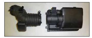
7. Loosen the hose clamp and then remove the intake hose from mass air sensor housing.
