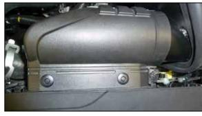
20. Install the fresh air scoop onto the heat shield and secure with the factory retaining pins.
