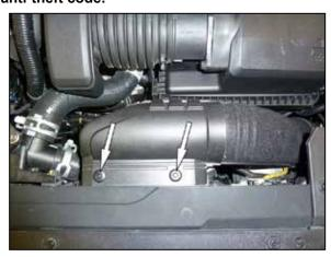
2. Push in the center of the retaining pins and then remove the fresh air retaining pins. Remove the fresh air intake scoop and duct from the vehicle.
