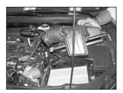
10. Unclip the air cleaner cover and remove the complete upper air cleaner assembly as shown.
