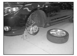
19. Raise the vehicle up and support it with jack stands, then, remove the front tire as shown.
