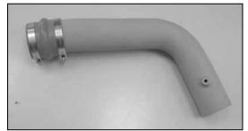
32. Install the silicone hose and hose clamps onto the cold air tube as shown.
