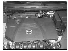
44. Reinstall the engine cover as shown.
