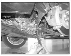
21. Remove the three plastic rivets and six hex bolts on the inner wheelhouse valance, then, pull the inner wheel house valance downward as shown. 24. Install the silicone hose and hose clamps onto the throttle body as shown.
