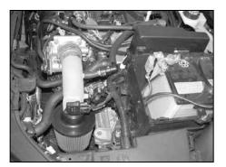
45. This K&N<sup>®</sup> high flow intake system has been designed to be used in two different configurations. In the case of inclement weather, the cold air tube can be removed and the air filter can be clamped onto the intake tube located in the engine compartment to avoid the possibility of ingesting water into the engine.
