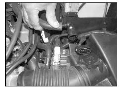
6. On vehicles equipped with a quick release crankcase vent hose fitting, release the fitting and disconnect the crankcase vent hose from the intake tube. On vehicles not equipped with a quick disconnect fitting, unplug the crankcase vent fitting from the intake tube. 8. Loosen the hose clamp at the throttle body as shown.
