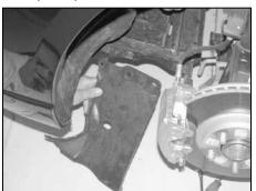
20. Remove the four bolts and one plastic rivet from the inner valance then, remove the valance as
