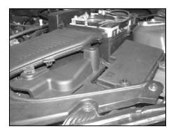
4. Slide the battery cold air vent backwards and remove from the engine compartment as shown.
