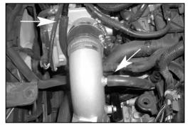
30A. On vehicles not equipped with the crankcase quick disconnect fitting, install the provided silicone vent hose onto the factory plastic crankcase vent tube and then route it under the K&N<sup>®</sup> intake tube and connect the open end onto the K&N<sup>®</sup> intake tube as shown.
