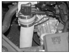
35. Slide the cold air tube onto the short ram tube as shown.
