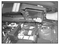
3. Disengage the plastic rivet as shown.
