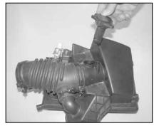
14. Remove the mass air sensor from the air cleaner cover as shown.
