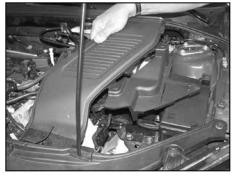
42. Slide the vent into the core support and line up the other end with the battery box and secure with plastic rivet.
