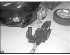
22. Remove the three bolts that secure the air intake resonator to the inner fender, then, remove the resonator as shown.
