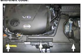
2. Remove the three bolts that secure the fresh air intake duct shown. These bolts will be re-used in a later step.
