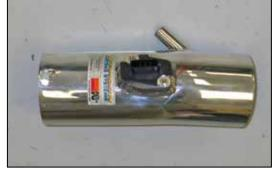
19. Install the mass air sensor into the K&N $^{\! \rm 8}$  intake tube and secure with the provided hardware.
