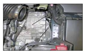
8. Remove the two air filter housing mounting grommets shown.
