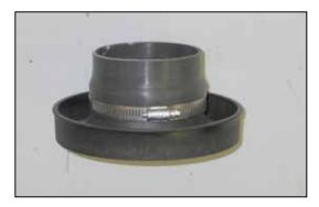
24. Install the silicone hose (084091) onto the air filter adapter and secure with the provided hose clamp as shown.
