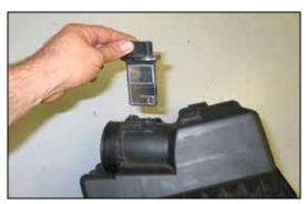
18. Remove the two screws securing the mass air sensor, and then remove the mass air sensor from the stock air box as shown.
