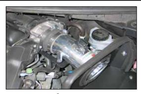
21. Install the K&N® intake tube into the silicone hose installed onto the throttle body and align it with the tube mounting bracket. Secure the intake tube with the hardware and hose clamp provided.
