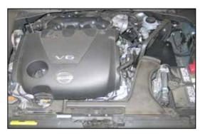
17. Re-install the fresh air intake duct onto the core support and into the heat shield and secure with the factory bolts.
