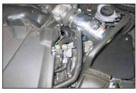
23. Install the crank case vent hose into the factory crank case vent hose and then connect the open end onto the K&N® intake tube as shown.
