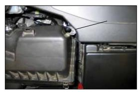
Remove the air box retaining bolt shown.
