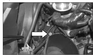
16. Place the provided spacer onto the front mounting point of the original air cleaner cover as shown.
