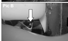
24. Slide the K&N® cold air tube into the silicone hose on the K&N® short ram tube (Pic. A) and line up the bracket with the rubber mounted stud (Pic. B) and secure with the provided hardware as shown.
