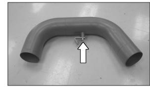
22. Install the angle bracket onto the K&N<sup>®</sup> cold air tube in the orientation shown, but do not tighten completely at this time.
