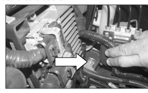
5. Remove the ground wire from the rear bracket on the ABS pump as shown.
