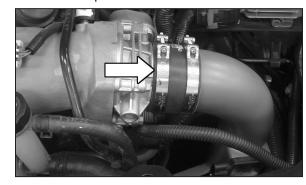
18. Slide the silicone hose onto the throttle body, but do not tighten at this time.
