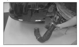
13. Loosen the hose clamp that secures the air inlet duct to the lower air cleaner assembly, then, loosen and remove the bolt that secures the air inlet duct and remove the air inlet duct as shown.
