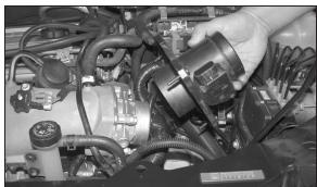
4. Loosen the three screws to remove the stock air cleaner cover as shown.
