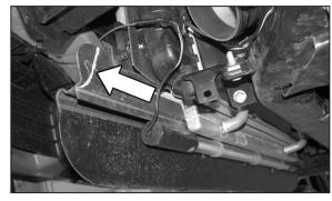
21. Trim the top side of the air deflector for tube clearance if needed.
