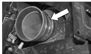
19. From underneath the vehicle install the silicone hose and hose clamps onto the K&N® short ram tube as shown.
