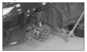
10. Jack the vehicle up and support it with jack stands, then, remove the front driver side tire as shown.
