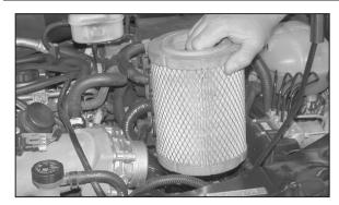
9. Remove the air filter from the lower air cleaner assembly as shown.
