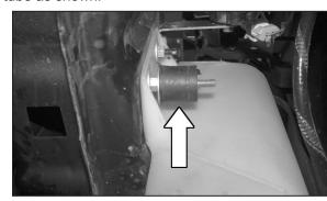
20. Install the provided washer and the provided rubber mounted stud onto the lower bolt on the windshield wiper reservoir as shown.
