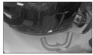
23. From underneath the vehicle slide the K&N<sup>®</sup> cold air tube up into the inner fender as shown.
