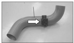
14. Install the mass air sensor into the K&N $^{\circ}$  short ram tube using the stock bolts removed in step five.
