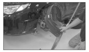
11. Remove the eight plastic rivets and two screws, then lower the inner fender valance downward as shown.
