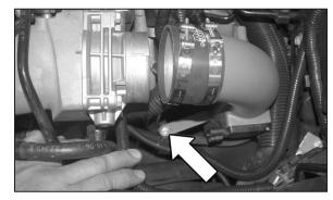
17. Slide the tube through the inlet of the lower air cleaner assembly, then, line up the bracket with the spacer/threaded hole and secure with the bolt removed in step 8.
