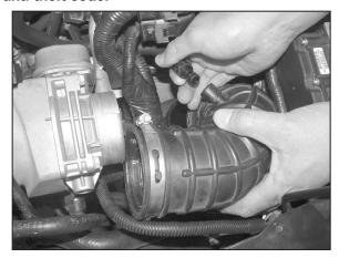
2. Loosen the stock hose clamps and pull the stock hose off the throttle body and the air cleaner, then, disconnect the crank case vent hose to remove the stock intake hose.
