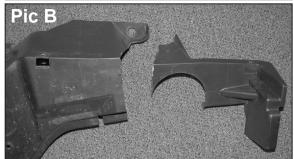
30. Cut out the provided template and place onto the plastic valance and mark the trim lines (Pic. A) then cut the valance as shown, (Pic. B).
