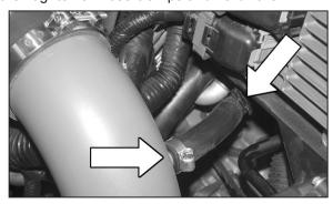
28. Slide the provided hose and hose clamp onto the original crank case vent hose, then, connect the other end to the vent on the K&N® short ram tube and secure with the provided hose clamp as shown.
