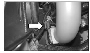
33. Reconnect the mass air sensor electrical connection as shown.
