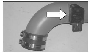
15. Install the provided silicone hose and hose clamps onto the K&N® short ram tube as shown.
