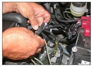
11. Remove the tape that binds the three wire harnesses together.
