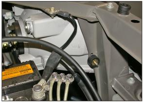
19. Install the provided rubber mounted stud into threaded hole on the radiator core support from step 8.
