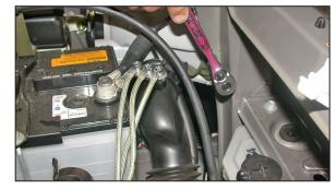
8. Loosen and remove the bolt that secures the air inlet tube to the radiator core support as shown.
