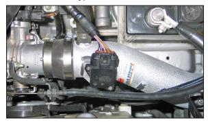
29. Reconnect the mass air sensor electrical connection as shown.
