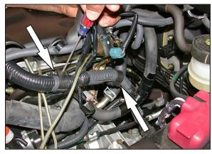
12. Unclip the two plastic wire harness clips and slide the wire harness forward to gain more slack for the mass air sensor electrical connection as shown.
