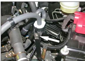
18. Slide the PWM vacuum switching valve onto the "L" bracket from the previous step. NOTE: On the '06 & later models, using the supplied washer and bolt, secure the PWM vacuum switching valve to the "L" bracket as shown.
