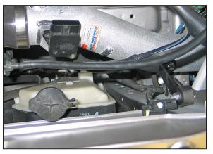
26. Adjust the tube for best fit then tighten the bracket and the hose clamp as shown.
