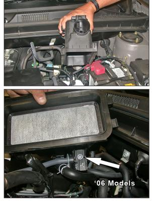
6. Release the clamps on the upper air cleaner assembly, then, remove the upper air cleaner assembly as shown.
