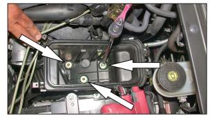
7. Remove the three screws that secure the lower air cleaner assembly as shown.
