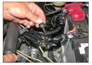
10. Remove the plastic wire harness clip that secures the mass air wire to other miscellaneous wires as shown.
