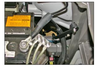
9. Pull upwards to remove the lower air cleaner assembly as shown.
