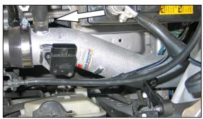
28. Slide the hose mender into the stock crank case vent hose, then, connect the other end to the vent on the K&N<sup>®</sup> Typhoon<sup>®</sup> cold air tube as shown.
