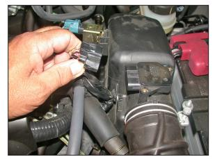
2. Disconnect the mass air sensor electrical connection and unclip the wire harness from the side of the air cleaner assembly as shown. **NOTE: On '06 & later models, unclip the MAS** wiring harness from air box lid.
