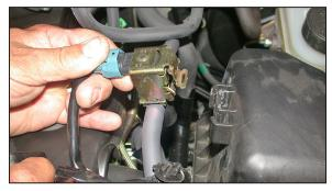
3. Pull firmly upwards to remove the PWM vacuum switching valve from the side of the air cleaner assembly as shown.
