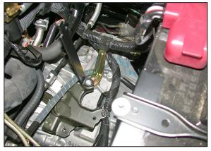
17. Using the provided hardware secure the provided large "L" bracket to the original air cleaner mounting bracket as shown.
