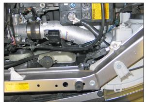
24. Rotate the end of the K&N<sup>®</sup> Typhoon<sup>®</sup> intake tube downward, then slide the other end of the tube into the silicone hose on the throttle body as shown
