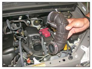
5. Loosen the hose clamps at the throttle body and at the air cleaner assembly, then, remove the stock intake tube as shown.
