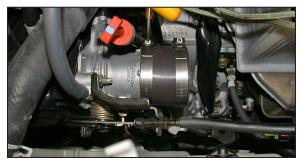
16. Install the silicone hose and hose clamps onto the throttle body and tighten as shown.
