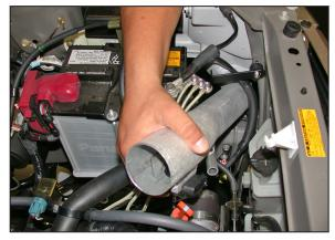
23. Slide the K&N<sup>®</sup> Typhoon<sup>®</sup> cold air tube into the area directly below the headlight as shown.
