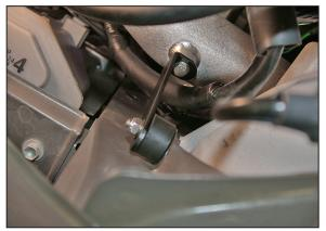
25. Line up the bracket from step 20 with the threaded boss on the K&N<sup>®</sup> Typhoon<sup>®</sup> cold air tube, then secure it using the provided hardware as shown, but do not tighten at this time.
