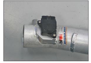
22. Install the stock mass air sensor into the K&N<sup>®</sup> Typhoon<sup>®</sup> cold air tube and secure with the provided hardware as shown.
