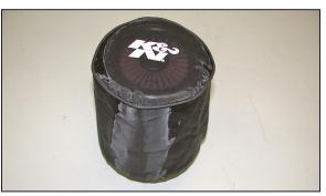
30. Install the K&N<sup>®</sup> Drycharger onto the K&N<sup>®</sup> Air filter as shown.
