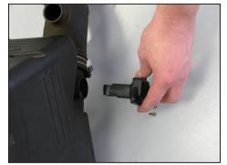
15. Remove the two screws that secure the mass air sensor into the stock air box; then, remove the mass air sensor.
