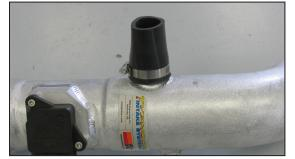
17. Install the provided silicone hose (084074) onto the K&N^ $^{\mbox{($n$)}}$  intake tube and secure with the provided hose clamp.
