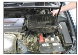
8. Remove the lower air box from it's place of attachment as shown in the photograph. NOTE: K&N Engineering, Inc., recommends that customers do not discard factory air intake.
