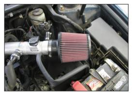
25. Install the K&N<sup>®</sup> air filter onto the intake tube; secure with the provided hose clamp. NOTE: Drycharger<sup>®</sup> air filter wrap; part # RX-4990DK is available to purchase separately. To learn more about Drycharger<sup>®</sup> filter wraps or look up color availability please visit http://www.knfilters.com<sup>®</sup>.
