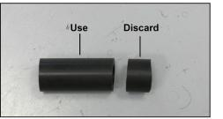
18. Cut the provided silicone hose (08415) hose from 2-3/8" (as supplied) to 1-3/4" long as shown in the photograph.
