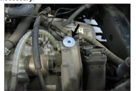
11. Place the provided rubber washer and fender washer onto the lower air box mount as shown in the photograph.
