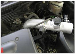
21. Install the K&N<sup>®</sup> intake tube into the silicone (084016) hose on the throttle body; and align with the intake tube mounting bracket which was installed in step 13.
