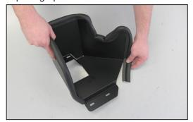
10. Install the provided edge trim onto the heat shield as shown in the photograph. NOTE: Some trimming of the edge trim may be necessary.
