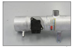
16. Install the mass air sensor into the  $K\&N^{\mbox{(R)}}$  intake tube and secure with provided hardware.
