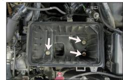
2. Disconnect the mass sensor electrical connection by depressing the center tab and gently pulling the harness away from the mass air sensor.
