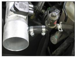
23. On vehicles equipped with an "EVAP canister closed valve", install the "EVAP canister closed valve" into the silicone hose which was installed in step 19; secure with the provided hose clamp.
