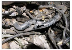
9. Using the provided tie wrap, secure the heater hose to the throttle body bypass hoses as shown in the photograph.
