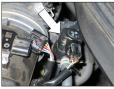
6. Lift up and remove the EVAP solenoid from the rear of the factory intake tube.
