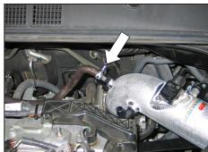
25. On vehicles equipped with EVAP valve, attach the EVAP vent line to the straight fitting installed in the  $K\&N^{\otimes}$  intake tube.
