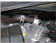
5. Disconnect the EVAP vent line from the factory intake tube as shown.
