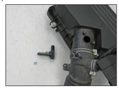
21. Remove the mass air sensor from the factory upper air box.
