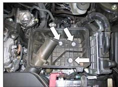
9. Remove the three lower air box mounting bolts and then remove the lower air box housing from the vehicle.
