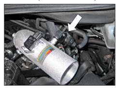
24. On vehicles equipped with EVAP valve, attach the EVAP solenoid to the bracket installed onto the K&N® intake tube and secure with the factory screw.
