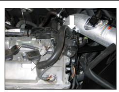
26. Attach the provided crank case vent hose to the  $90^{\circ}$  vent fitting in the K&N® intake tube and to the valve cover port as shown.
