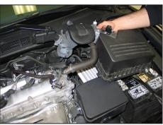
8. Loosen the hose clamp that secures the factory intake tube to the throttle body and then remove the intake tube and upper air box assembly.
