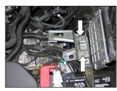
Remove the two air box mounting bracket bolts and then remove the bracket from the vehicle.
