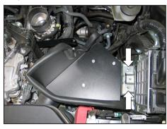
18. Install the heat shield assembly into the vehicle and secure with the factory air box mounting bracket bolts.
