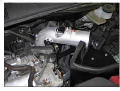
23. Install the K&N® intake tube into the silicone hose at the throttle body and align with the mounting bracket previously installed. Secure the tube with the provided hose clamp and hardware.
