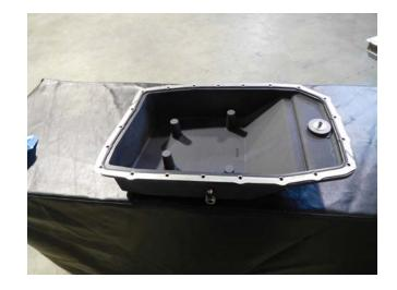
5. Clean the transmission mounting surface and install the B&M pan onto the transmission with the supplied M6 allen bolts and washers, qty. 21. Torque pan bolts to factory torque specs. Then follow your stock re-fill procedure. **NOTE:** Make sure transmission filter is pushed up into place inside the transmission.
