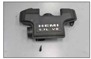
23. Remove the inlet temperature sensor from the intake plenum and then remove the O-ring from the sensor.
