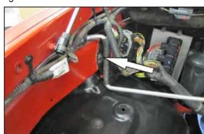
12. Remove the bolt show which secures the ECU harness bracket to the inner fender.
