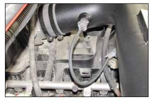
28. Connect the provided extension harness to the factory inlet air temperature sensor harness and then connect the open end to the sensor installed into the K&N® intake tube.
