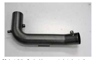
20. Install the final rubber mounted stud onto the intake tube as shown.
