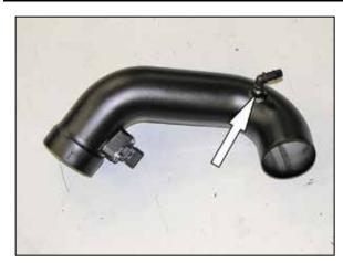
20. Install the provided 90° vent fitting into the K&N® intake tube as shown.
