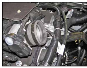
17. Install the provided step coupler (08186) onto the throttle body and secure with the provided hose clamp.
