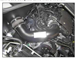
21. Install the K&N® intake tube into the hump coupler and then into the step coupler at the throttle body, adjust the tube for best fit and then secure with the provided hose clamps.
