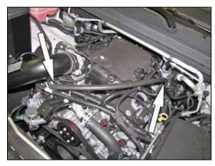
23. Install the crank case vent hose onto the fitting installed into the K&N® intake tube and then connect the hose mender into the fitting on the valve cover.
