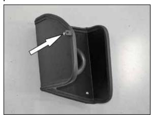
13.Install the provided heat shield mounting bracket (07805) onto the heat shield as shown using the provided hardware.
