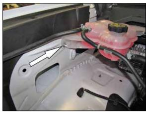
14. Remove the nut that secures the front of the coolant reservoir.
