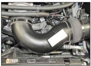
24. Install the K&N<sup>®</sup> intake tube into the hump coupler and then into the coupler at the throttle body, adjust the tube for best fit and then secure with the provided hose clamps.
