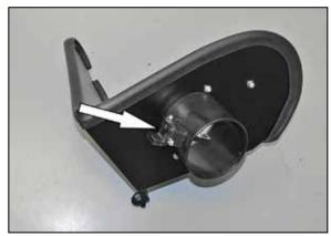
19. Install the mass air sensor into the K&N<sup>®</sup> mass air housing and secure with the provided hardware.
