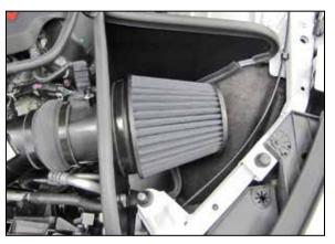
27. Install the K&N<sup>®</sup> air filter and secure with the provided hose clamp.
