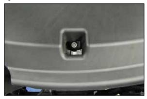
4. Remove the front center bolt securing the intake plenum to the engine and remove the plenum from tthe vehicle.
