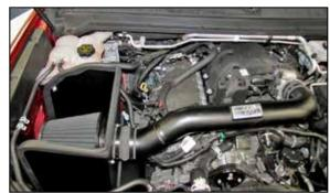
22. Reconnect the vehicle's negative battery cable. Double check to make sure everything is tight and properly positioned before starting the vehicle.
