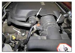
2. Loosen the hose clamp that secures the intake hose to the air filter housing. Using a screwdriver, unlock the small clamp that secures the vent line to the connector and then disconnect the vent line. Remove the bolt securing the intake plenum to the engine.
