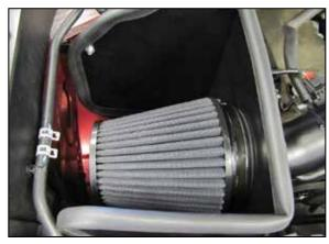
21. Install the K&N<sup>®</sup> air filter onto the filter adapter and secure with the provided hose clamp.
