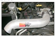
21. Install the K&N® intake tube into the silicone hose at the throttle body and position so that the mounting bracket aligns with the plenum mounting location. Then secure with the provided hardware.
