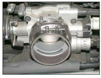
15. Install the provided silicone hose (084031) onto the throttle body and secure with the provided hose clamp as shown.
