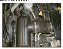
2. Loosen the hose clamp at the throttle body and the airbox mounting nut and then disconnect the crankcase vent hose from the inline fitting.
