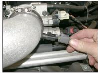
22. Reconnect the air temperature sensor electrical connection as shown.
