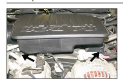
5. Loosen and remove the two intake plenum mounting bolts indicated.
