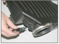
16. Twist the air temperature sensor counter clockwise and remove it from the stock intake
