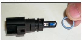
18. Remove the O-ring from the air temp. sensor as shown.
