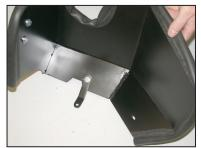
10. Install the "L" bracket (010122) onto the heat shield with the provided hardware as shown.
