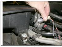
4. Depress the locking tab on the air temperature sensor electrical connection and then pull to disconnect he sensor electrical connection.
