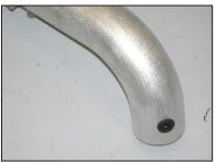
17. Install the provided grommet into the  $K\&N^{\circledcirc}$  intake tube as shown.
