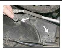
13. Install the two threaded inserts into the airbox mounting grommet locations as shown.
