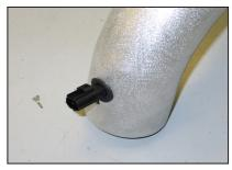
19. Install the sensor into the grommet installed in step #17.
