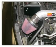
26. Install the air filter assembly onto the K&N® intake tube and secure with the provided hose clamp as shown.
