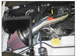
35. The C.A.R.B. exemption sticker, (attached), must be visible under the hood so that an emissions inspector can see it when the vehicle is required to be tested for emissions. California requires testing every two years, other states may vary.
