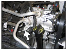
10. Remove the lower rear A/C compressor mounting bolt shown. **NOTE: This bolt will be reused in the next step.**
