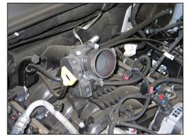
9. Install the silicone hose (084036) onto the throttle body and secure with the provided hose clamp.
