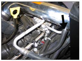
30. Connect the provided silicone vent hose to the modified factory vent tube and then connect the open end to the K&N<sup>®</sup> intake tube as shown.
