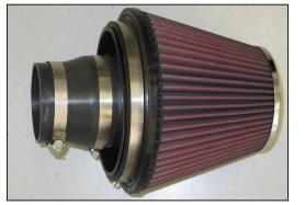
32. Install the provided silicone hose (084055) onto the filter assembly and secure with the provided hose clamp.
