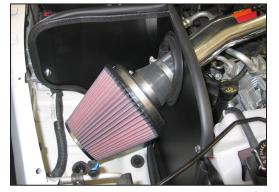
33. Install the filter assembly onto the K&N<sup>®</sup> intake tube and secure with the provided hose clamp.
