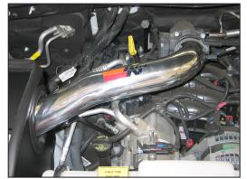
28. Install the K&N<sup>®</sup> intake tube into the silicone hose at the throttle body and align with the tube mounting bracket installed during step #11. Secure the intake tube with the provided hose clamp and hardware.
