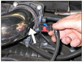
23. On vehicles equipped with and inlet air temperature sensor, install the K&N<sup>®</sup> intake tube into the silicone hose at the throttle body. Position the inlet air temperature sensor electrical connection for best fit. Mark the location for drilling.
