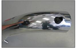
27. Install the air temperature sensor into the grommet installed into the K&N $^{\circ}$  intake tube as shown.
