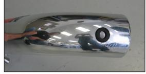
26. Install the supplied grommet into the K&N<sup>®</sup> intake tube as shown.
