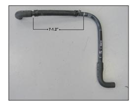
7. Using a knife, cut the crank case vent hose 7-1/2" from the valve cover elbow fitting as indicated.
