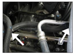
25. Install the crankcase vent hose onto the NPT fitting on the K&N<sup>®</sup> intake tube. Install the hose mender end into the factory elbow on the valve cover.
