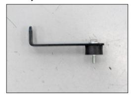
11. Install rubber mounted stud onto the heat shield mounting bracket (070952) as shown using the provided hardware.
