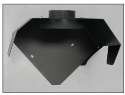
9. Attach the filter adapter into the heat shield as shown, and secure with the provided hardware.
