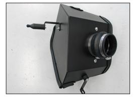
15. Install the bracket/stand-off assembly onto the heat shield using the hardware provided as shown.
