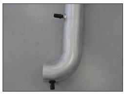
22. Install the inlet air temperature sensor into the grommet previously installed during step #21. **NOTE: The inlet air temperature sensor is very fragile, use care when installing the sensor.**
