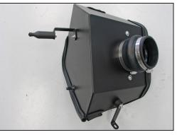
16. Attach the short standoff assembly to the heat shield and secure with the provided hardware as shown.
