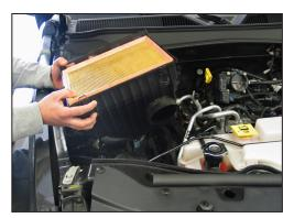
7. Lift up the lower airbox assembly to dislodge it from the mounting grommets, then disconnect the fresh air duct from the lower airbox and then remove the lower airbox from the vehicle.
