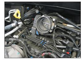
2. Release the red locking tab and then disconnect the inlet air temp sensor electrical connection.
