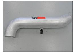
19. Install the provided NPT vent fitting into the  $K\&N^{\mbox{\tiny B}}$  intake tube as shown.
