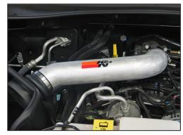
23. Install K&N<sup>®</sup> intake tube into the silicone hose at the filter adapter and then into the silicone hose on the throttle body. Secure the intake tube with the provided hose clamps.
