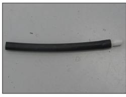
24. Install the provided hose mender into the provided crankcase vent hose as shown.
