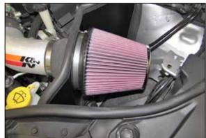
25. Install the K&N® air filter and secure with the provided hose clamp.
