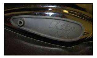
26. During inclement weather such as rain or snow, On Jeep grand Cherokee's Install the provided heat extractor block off (21575) into the vent of the hood to reduce the chance of unwanted water and or snow contacting the K&N® air filter.
