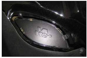
28. Place the provided block off into position and reinstall the factory screws.
