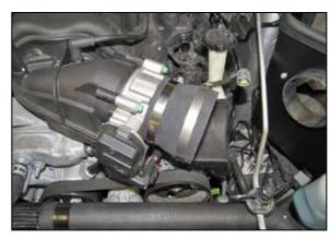
17. Install the step coupler (08497) onto the throttle body and secure with the provided hose clamp.
