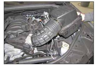
6. Lift up the air filter assembly to dislodge it from the mounting grommets and the remove the complete assembly from the vehicle.
