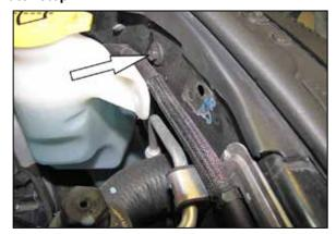
Remove the core support bolt shown.NOTE: This bolt will be reused in the next step.
