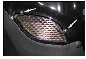
27. Some Dodge Durango models may be equipped with heat extractor vents in the hood. During inclement weather or driving in wet conditions, K&N® recommends installing the provided heat extractor block off plate. Remove the two screws that secure the factory grid in position.
