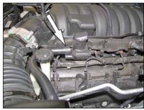
4. Disconnect the crank case vent hose from the valve cover port.
