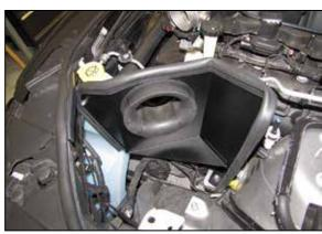
16. Install the heat shield assembly into the vehicle so the mounting grommet slides onto he inner most mounting stud. Align the heat shield with the mounting bracket and then secure with the spacer and hardware provided.
