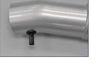
16. Install the provided grommet into the K&N<sup>®</sup> intake tube then remove the O-Ring from the inlet air temperature sensor and then install the sensor into the grommet install into the K&N<sup>®</sup> intake tube. **NOTE: The inlet air temperature sensor is very fragile, use care while handling the sensor.**
