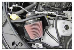
14. Install the heat shield/Air filter assembly onto the air filter housing mounting studs as shown.
