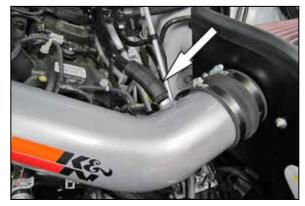
21. Install the provided crank case vent hose onto the fitting installed into the K&N<sup>®</sup> intake tube and then connect the other end to the factory crank case vent tube.
