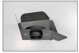
10. Install the filter adapter into the K&N<sup>®</sup> heat shield and secure with the provided hardware as shown.
