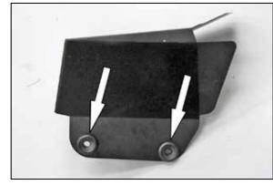
9. Install the two mounting grommets from the previous step into the K&N<sup>®</sup> heat shield as shown.
