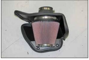
13. Install the K&N<sup>®</sup> air filter onto the filter adapter and secure with the provided hose clamp. NOTE: Drycharger<sup>®</sup> air filter wrap; part # RF-1042DK is available to purchase separately. To learn more about Drycharger<sup>®</sup> filter wraps or look up color availability please visit http://www.knfilters.com<sup>®</sup>.
