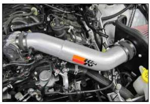
19. Install the K&N<sup>®</sup> intake tube into the coupler at the throttle body and then into the hump coupler, adjust the tube for best fit and then secure with the provided hose clamps.
