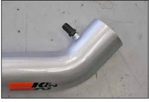
17. Install the provided vent fitting into the  $K\&N^{\otimes}$  intake tube as shown.
