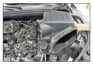
7. Lift up the air filter housing to dislodge it from the mounting grommets and then remove it from the vehicle.
