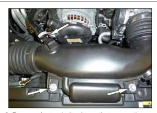
3. Remove the two bolts shown that secure the intake tube to the core support. Push the white locking for the crank case vent line down and then disconnect the crank case vent line from the intake
