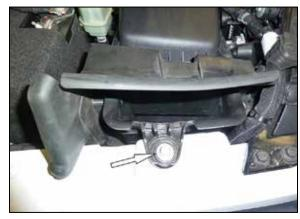
4. Remove the bolt shown that secures the fresh air intake duct to the fender, then lift and remove the complete intake system from the vehicle.
