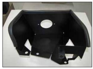
4. Install the provided edge trim onto the heat shield as shown.
