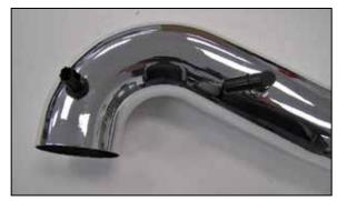
11. Install the inlet air temperature sensor into the  $K\&N^{\odot}$  intake tube using the provided grommet. Install the 90° NPT fitting onto the  $K\&N^{\odot}$  intake tube as shown.
