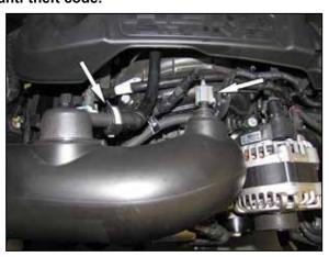
2. Disconnect the inlet air temperature sensor electrical connection and crank case vent line from the factory intake tube.
