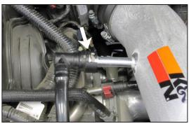
21. Connect the crankcase vent hose to the quick connect fitting on the K&N® intake tube as shown.
