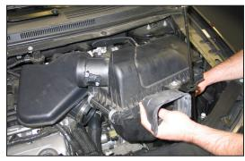
6. Remove the airbox from the vehicle.
