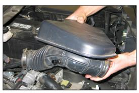
7. Loosen the hose clamp which secures the stock intake tube to the throttle body and then remove the intake tube from the vehicle.
