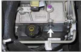
9. Remove the transmission pan bolt shown.
