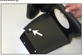
12. On 2007 and 2008 model vehicles, install the "L" bracket (070066) onto the heat shield using the provided hardware as shown.
