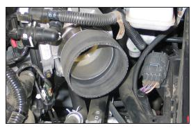
15. Install the silicone hose (08051) onto the throttle body and secure with the provided hose clamp.
