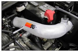
19. Install the K&N® intake tube into the silicone hose at the throttle body and align with the mounting bracket installed in step #10. Secure the intake tube with hose clamp and hardware provided.
