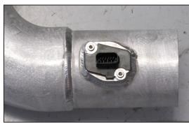
17. Install the mass air sensor into the K&N® intake tube and secure with the provided screws.
