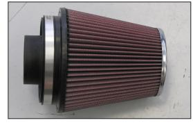
22. Install the filter adapter into the K&N® air filter and secure with the provided hose clamp.
