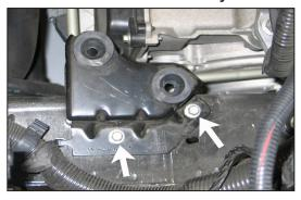
8. Remove the two bolts which secure the airbox mounting bracket to the inner fender.
