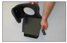
11. Install the provided edge trim onto the heat shield as shown.
