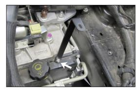
10. Install the intake tube mounting bracket (070095) onto the transmission pan and secure with the factory bolt removed in step #9.
