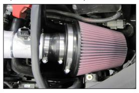
24. Install the filter assembly onto the intake tube and secure with the provided hose clamp.
