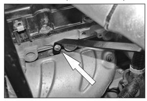
19. Attach the tube-mounting bracket to the engine using the provided hardware as shown.
