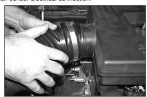
3. Loosen the hose clamp that retains the stock intake tube to the resonator, and then remove the tube from the resonator as shown.
