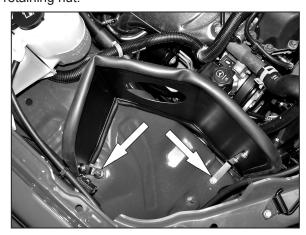
14. Install the heat shield into the vehicle using the hardware provided and the factory air box retaining nut.
