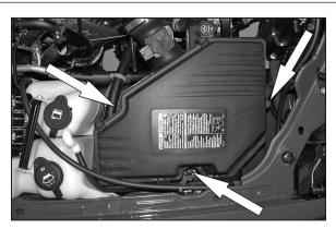
4. Loosen the two air box retaining bolts and one retaining nut.
