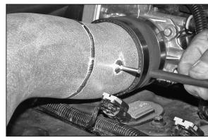
20. Install the provided 4mm vacuum hose onto the fuel pressure regulator, then onto the vent fitting on the  $K\&N^{\circledcirc}$  intake tube.
