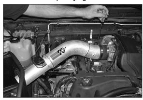
18. Install the K&N® intake tube into the silicone hose at the throttle body and through the heat shield, secure with the provided hose clamp.
