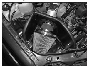
24. Install the air filter assembly onto the K&N® intake tube and secure with the provided hose clamp.
