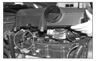
8. Remove the intake resonator from the engine as shown.
