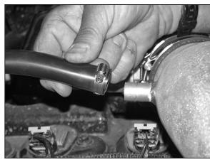
21. Install the provided crankcase vent hose onto the valve cover, then onto the K&N® intake tube as shown.
