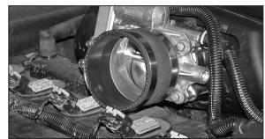
9. Install the silicone hose (08051) onto the throttle body and secure with the provided hose clamps as shown.
