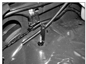
13. Install the "L" bracket (070602) onto the stock air box-mounting stud using the factory air box-retaining put
