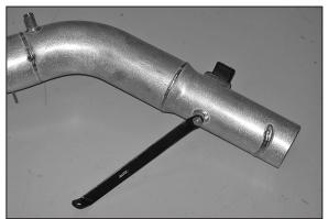
17. Install the small end of the tube-mounting bracket on the K&N<sup>®</sup> intake tube as shown.
