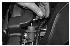
6. On vehicles equipped with a fuel pressure regulator disconnect the fuel pressure regulator vacuum hose from the fuel pressure regulator as shown.
