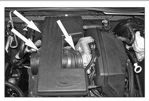
7. Loosen the two bolts that retain the intake resonator to the engine, and then loosen the hose clamp at the throttle body.
