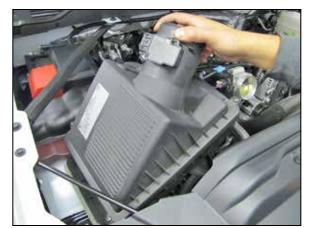
6. Lift up the air box to dislodge it from the mounting grommets, and then remove it from the vehicle as shown. **NOTE: K&N Engineering, Inc., recommends that**
