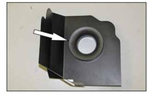
9. Install the provided filter adapter into the heat shield and secure with the provided hardware.
