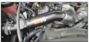
17. Install the K&N<sup>®</sup> intake tube into the coupling hoses and then adjust the tube for best fit. Secure the hoses and tube with the provided hose clamps.
