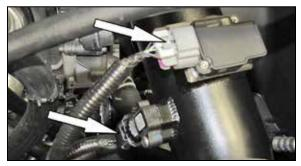
20. Reconnect the mass air sensor and humidity sensor electrical connections.
