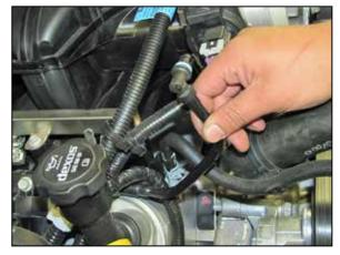
7. Release the locking ring and then disconnect the crank case vent tube from the valve cover vent port.
