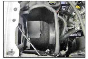
11. Install the heat shield assembly onto the air filter housing mounting plate location and secure with three of the factory bolts from step #8.
