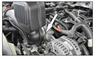
5. Loosen the hose clamps that secure the intake tube to the throttle body and air filter housing. Unhook the radiator hose clip from the intake tube and then remove the intake tube from the vehicle. customers do not discard factory air intake.
