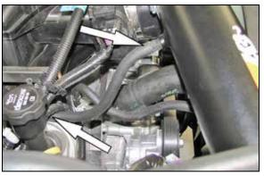
18. Install the provided crank case vent hose onto the fitting installed into the  $K\&N^{\odot}$  intake tube and then onto the valve cover port. Secure the hose to the valve cover port with the provided hose clamp.
