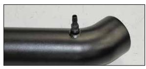
14. Install the provided vent fitting into the K&N<sup>®</sup> intake tube as shown.
