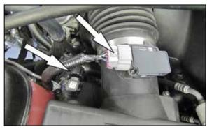
3. Disconnect the mass air sensor and humidity sensor electrical connections.
