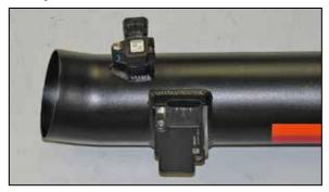
13. Install the mass air sensor and humidity sensors into the  $K\&N^{\textcircled{B}}$  intake tube and secure with the provided hardware.
