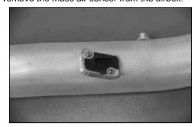
21. Install the mass air sensor into the K&N<sup>®</sup> intake tube and secure with the screws removed in step #20.
