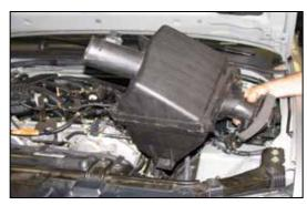
10. Pull firmly on the airbox to dislodge it from the mounting grommets and remove it from the vehicle. NOTE: K&N Engineering, Inc., recommends that customers do not discard factory air intake.
