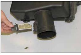
20. Remove the two screws, which secure the mass air sensor to the stock airbox and then remove the mass air sensor from the airbox.
