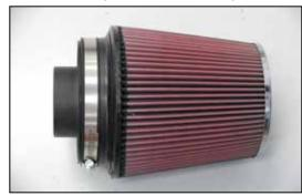
24. Install the filter adapter into the air filter as shown and secure with the provided hose clamp.
