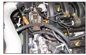
23. Attach the provided crank case vent hose to the valve cover and K&N<sup>®</sup> intake tube as shown and secure with the provided hose clamps.
