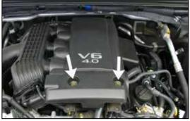
27. Reinstall the engine cover removed in step #4 and secure with the factory mounting bolts.
