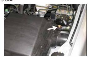
9. Remove the airbox retaining bolt shown.
