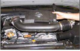
8. Remove the intake tube from the vehicle as
