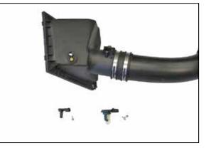
13. Remove the two sensors from the stock air filter housing.
