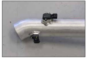
14. Install the sensors into the K&N<sup>®</sup> intake tube and secure with the provided hardware.
