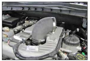
11. Install the provided coupler hose (08502) onto the turbo inlet and secure with the provided hose clamp. 15. Reconnect the mass air sensor and inlet air temperature sensor electrical connections.
