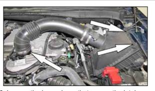
3. Loosen the hose clamp that secure the intake tube to the turbo inlet and then release the two clam shell clins that secure the upper air filter
