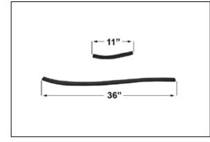
7. Cut the provided edge trim into two sections, one section will be 11" long and the section will be 36" long.
