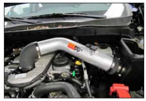
15. Install the K&N<sup>®</sup> intake tube into the coupler at the filter adapter and then into the hose at the turbo inlet, adjust the tube for best fit and then secure with the provided hose clamps.
