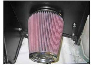
24. Install the K&N $^{\!0}$  air filter and secure with the provided hose clamp.
