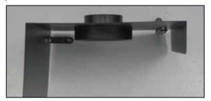
12. Install the filter adapter onto the heat shield and secure with the provided hardware.
