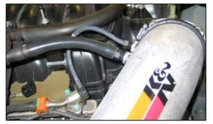
23. Connect the crank case vent hose and the fuel pressure hose to the fittings connected to the K&N® intake tube.
