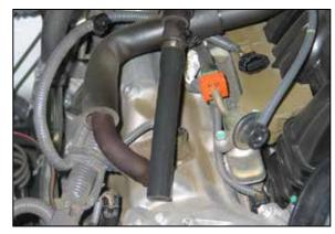
21. Install the crank case vent hose assembly into the factory crank case vent hose as shown.
