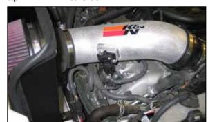
25. Reconnect the mass air sensor electrical connection.
