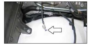
8. Remove the bolt securing the ground strap to the inner fender.
