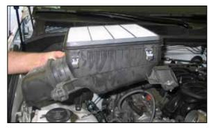
7. Loosen the two bolts securing the lower air box, and then remove the lower air box from the vehicle. NOTE: K&N Engineering, Inc., recommends that customers do not discard factory air intake.
