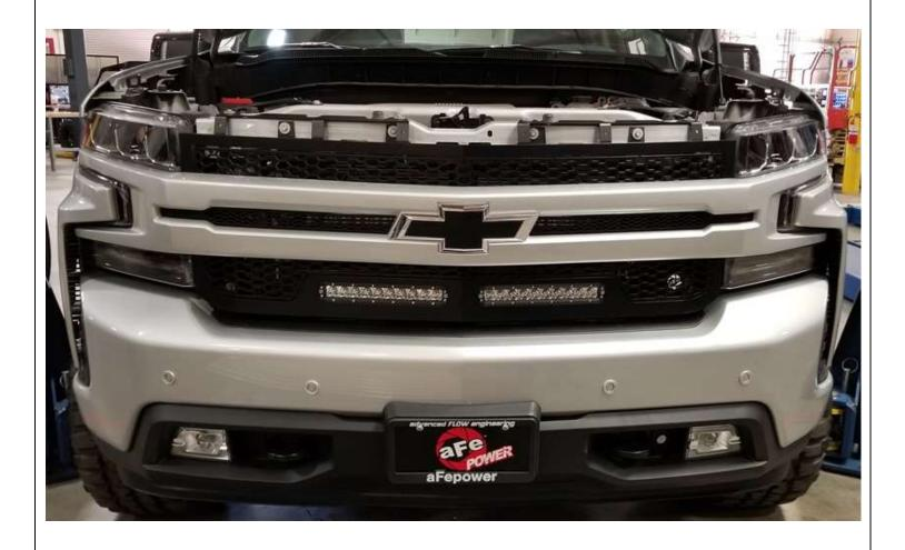
17. Place the aFe Scorpion grille assembly on the truck and attach the light wires to the 10" single row LED lights. Carefully push the attachment clips back into the core support (near the headlight and turn signals) attachment points.
