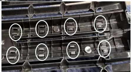
8. Disconnect the clips that secure the factory outer grille to the factory inner grille. Remove the factory inner grille and discard. Save the outer grille for reinstallation.
