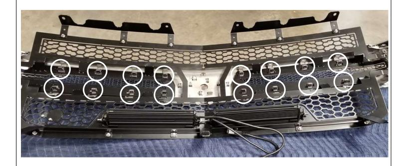
15. Install eight (8) supplied small fastener retaining clips onto the factory clip points protruding through the aFe Scorpion grille.
