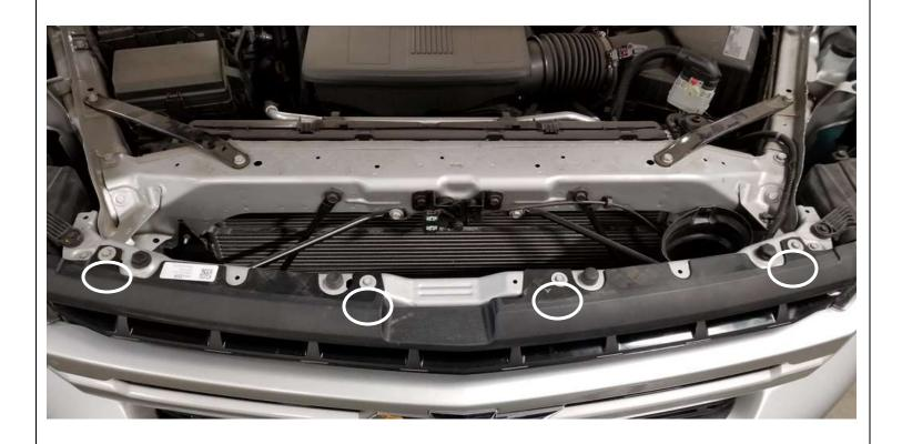
4. Remove the four (4) screws that retain the factory grille to the core support. Save the removed hardware for reinstallation.
