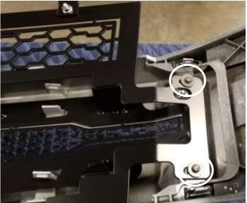
14. Install the four (4) screws removed in Step 7. Check the center line and tighten to factory specifacations.
