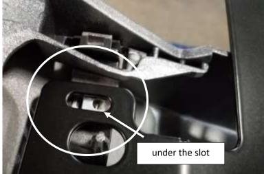
13. Install the two (2) supplied square aluminum spacers. Locate the slotted hole in the top left and right corners of the aFe Scorpion grille. The square aluminum spacers will be installed between the aFe Scorpion grille and the outer factory grille.
