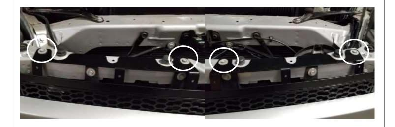
18. Install the four (4) screws that retain the grille to the core support that were removed in Step 4. Tighten to factory specifactions.
