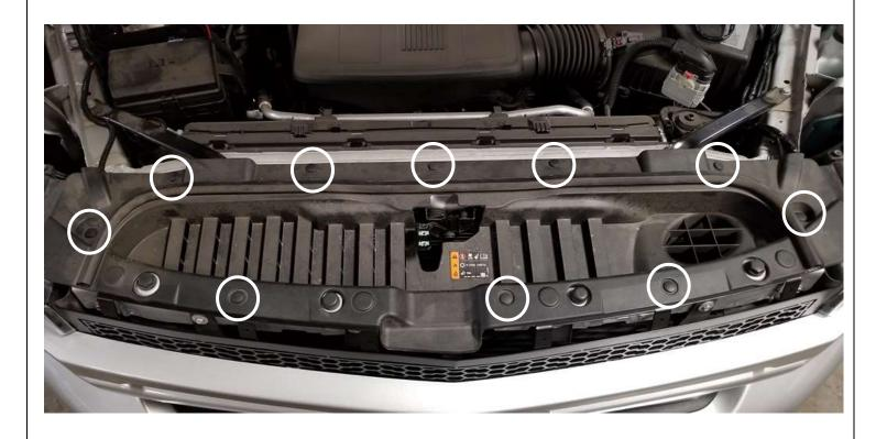
19. Reinstall the plastic radiator cover. Install the ten (10) push pin retainers that were removed in Step 3.
