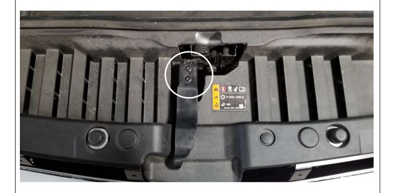
20. Reinstall the two (2) screws that attach the plastic handle to the hood release mechanism that were removed in Step 2. Tighten to factory specifications.
