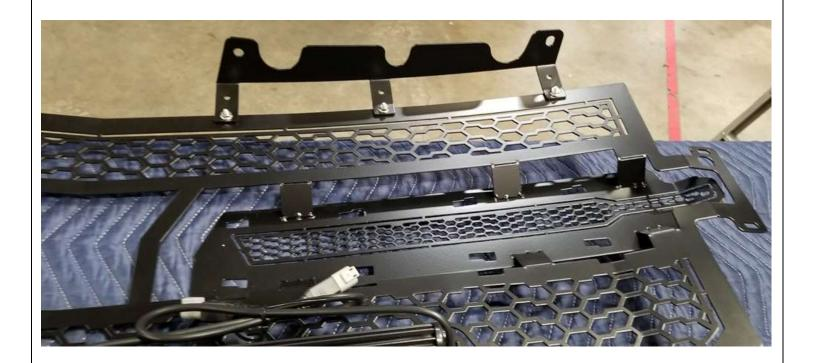
11. Install the one (1) supplied right top plate using three (3) #10-32 flange nuts.
