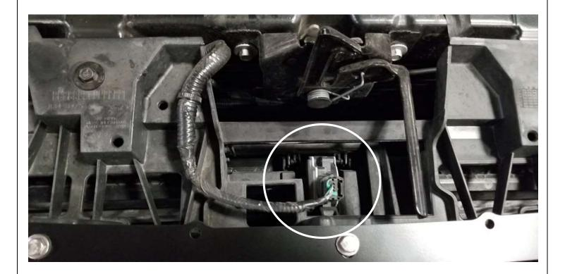
40. Reconnect the active shutter wiring connector.
