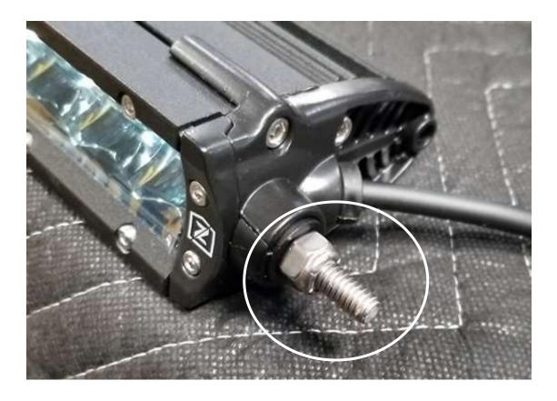
18. Remove and discard the two (2) nuts from the supplied 20" single row LED light.
