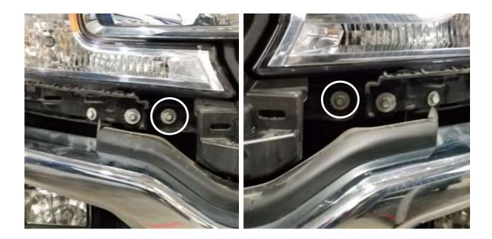
8. Remove the one (1) bolt located on each side of the grille. Save for reinstallation.
