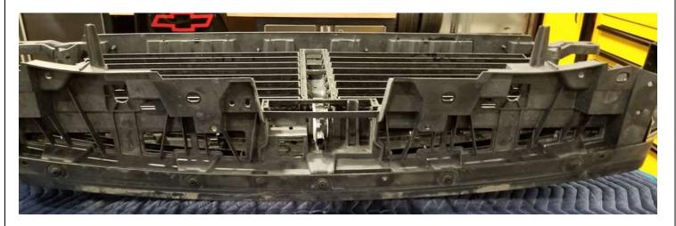
Note: To prevent scratching painted parts use protective covering between the grille and a <u>flat surface.</u>
