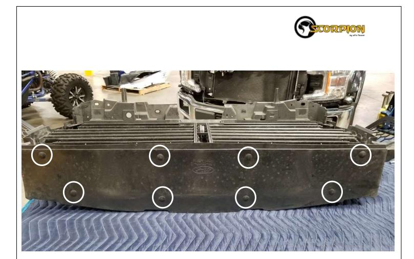
29. Reinstall the eight (8) push pins that attach the plastic lower shroud.
