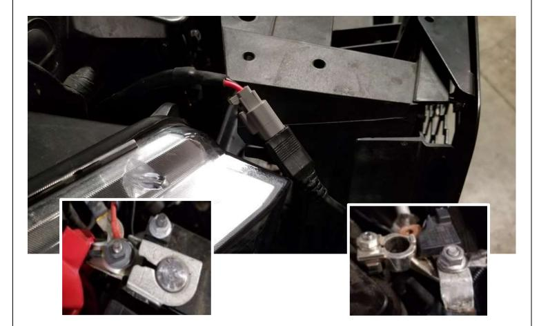
30. Before installing the aFe Scorpion grille, install the supplied power harness. The red wire goes on the positive battery terminal (+) and the black wire goes on the negative battery terminal (-). You will need to mount the switch inside the cab or to an available prewired switch. Use the (15) supplied 8" cable ties to secure the wiring loom to the vehicle.
