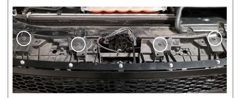
34. Install the grille assembly and install the four (4) factory screws removed in Step 4. Tighten to factory specifications.
