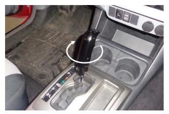
3. Thread the handle body all the way on to the shifter stick.
