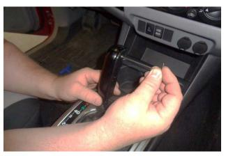
5. Install the left and right side plates (2) and (3) with the 4 flathead screws (4). (Two screws each side.)
