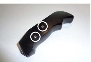
2. Thread the 4 set screws (Item 5) into the shifter handle body (1) until they are almost flush with the handle body. (Two screws each side.)
