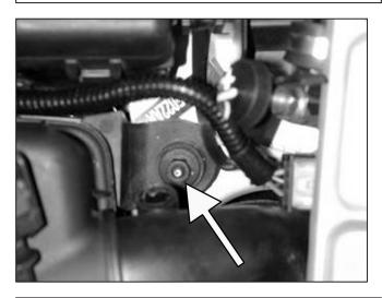
g. Loosen and remove nut holding down the air box. This nut is located by the vacant hole left by the IAT sensor.
