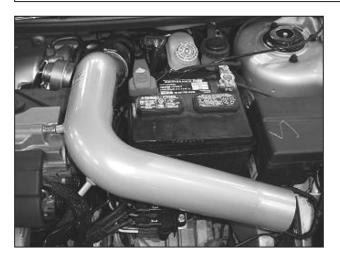
i. Insert the inlet pipe. Attach the coupler to the turbo and line up the bracket to the rubber mount.
