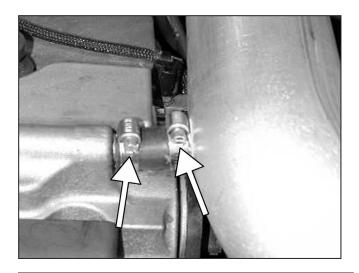
k. Attach the 1/2" diameter breather hose to the crankcase and inlet pipe. Make sure the nipples are inserted completely in the hose. Secure with provided hose clamps.
