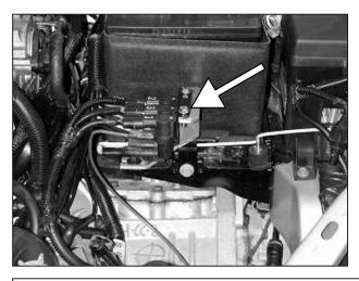
e. Secure the vacuum assembly to the vacuum assembly bracket. Make sure all the hard vacuum lines are clear of any obstruction.
