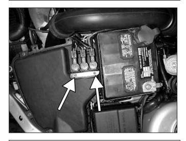
i. Remove the 2 screws holding down the vacuum assembly to the air box.
