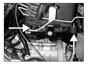
d. Insert rubber mount on the right side of the battery bracket. Attach the vacuum assembly bracket to the left side as shown. Secure the vacuum assembly bracket to the battery bracket.
