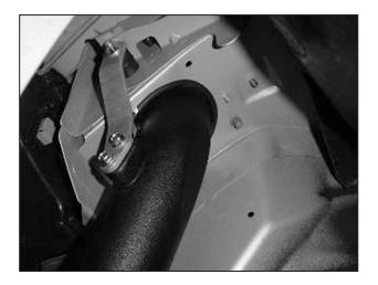
x. Secure the bracket on the rubber mount with a washer and nut.
