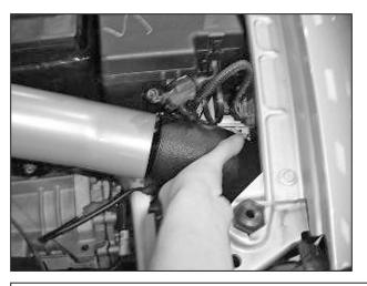
u. Insert the lower pipe from inside the fender.
