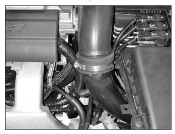
a. Loosen the hose clamp near the air box.
