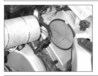
r. Attach the rubber edge trim to protect the lower pipe. Adhesive may be necessary.
