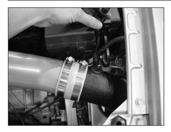
v. Attach the coupler and hose clamps. Make sure not to fully tighten the hose clamps. Make sure the IAT harness is clear.
