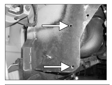
ac. Locate the two mounting holes in the fender.
