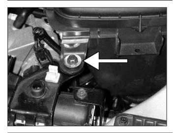
h. Remove the bolt holding down the air box to the radiator support.
