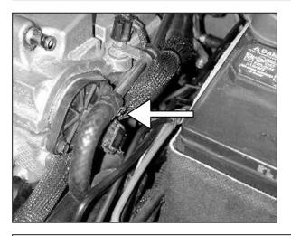
h. For more clearance, rotate the clip located near the crankcase vent so the tabs are directed towards the bottom of the car.
