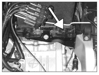
b. Loosen and remove the bolt on the right side of the battery bracket.
