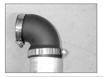
f. Attach the 3" side of the silicon elbow to the inlet pipe. Secure the elbow to the inlet pipe with the included hose clamp. The open end connects to the turbo inlet which sits horizontal. This opening is furthest away from the bracket.
