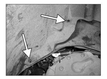
n. Remove the driver's side front wheel. Remove push in tabs from the fender liner. Do not throw away the fender liner hardware. They will be reused.
