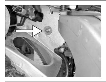
q. Secure the other side of the 1" rubber mount with the provided fender washer and nut.
