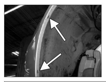
o. Remove the two TORX screws (T20) from the fender liner.
