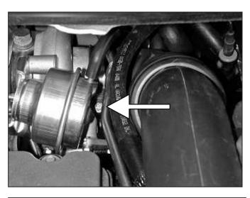
b. Loosen the hose clamp at the turbo inlet.
