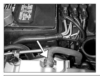
e. Remove the breather hose from the nipple on the valve cover. Check for oil, if present clean as necessary.
