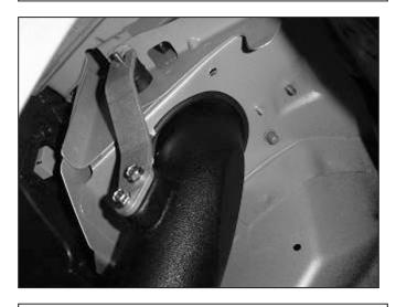
w. Line up the bracket with the 1" rubber mount from the inner fender side.
