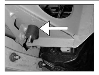
p. Locate this mounting hole inside the fender. Insert the 1" rubber mount.
