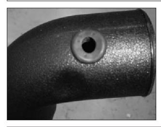
s. Insert the rubber grommet into the small hole in the plastic lower intake pipe.
