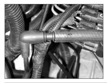
I. Insert the straight barded fitting into the vacuum cap from step 2d. Attach the 3/8" diameter breather hose to the other end of the barbed fitting.
