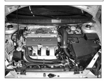
c. Remove the inlet air tube to the turbo.
