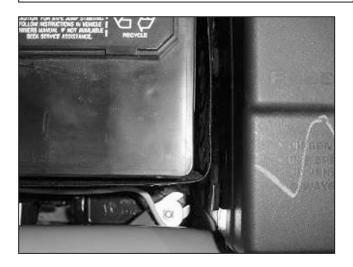
ab. There should be adequate clearance around both upper and lower pipes around the battery.
