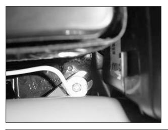
aa. Secure the upper inlet pipe to the 5/8" rubber mount on the battery tray. Check for clearance around the intake pipe.
