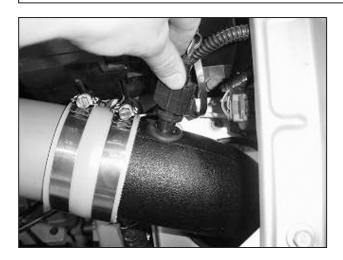
y. Carefully insert the IAT sensor into the rubber grommet on the lower intake pipe.
