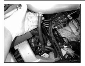
m. Secure the other end of the breather hose to the upper inlet pipe with the provided hose clamp.
