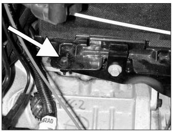
c. Loosen the bolt on the left side of the battery bracket.
