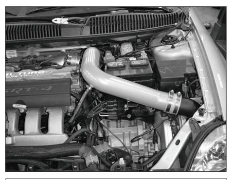
AEM® intake system installed
