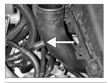
d. Unplug the vacuum cap at the base of the air box.
