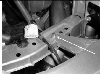
Fig. 9: Installation of the VSV for EVAP
