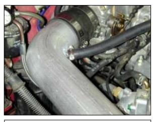
i. Attach the supplied ½" breather hose to the upper inlet pipe's nipple and the valve cover nipple. Secure each end of the breather hose with a ¾" hose clamp.
