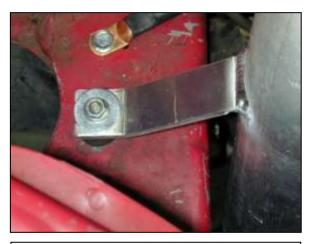
g. Install the lower inlet pipe. The inlet pipe's mounting bracket will line up with the rubber mount installed earlier. Secure in place with the supplied washer and M6 nut.
