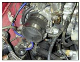
c. Install the supplied hose adapter onto the throttle body using the supplied #44 and #48 hose clamps. Use the #44 hose clamp on the throttle body side.
