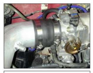
d. Attach the upper inlet pipe onto the hose adapter secured to the throttle body.
