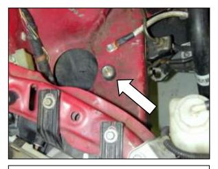
f. Install the supplied rubber mount into the hole in the engine compartment as shown. The hole is located in front of the passenger side shock tower where the stock airbox system was mounted.
