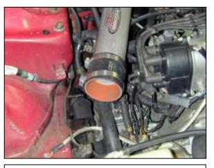
e. Install the supplied 3" coupler onto the upper inlet pipe as shown. Secure the coupler with a #48 hose clamp.
