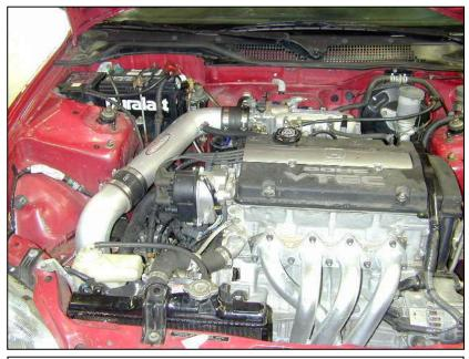
AEM® intake system installed
