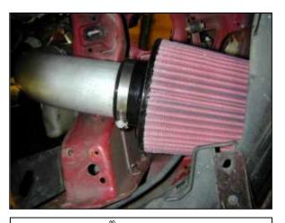
h. Install the AEM<sup>®</sup> air filter on the end of the inlet pipe. Once proper fitment is achieved, secure the air filter in place with the supplied hose clamp.
