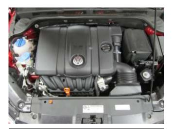
Factory air box system installed
