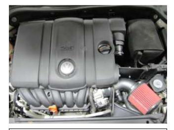
AEM<sup>®</sup> intake system installed
