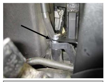
e) Using the supplied hardware, install the bolt, washer and spacer (1-1016 & 08275 & 07849) to attach the bracket to the post where the bolt was removed in 2f.
