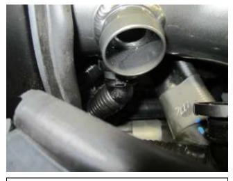
f) Before installing the tube into the hose at the throttle body, make sure to connect the lower (smaller) air injection connector onto the AEM tube. Note: Using warm soapy water on the O -ring (located in the connector) will help ease the connector onto the tube fitting. For models that do not have the larger connector, use the supplied cap to cap off the vent on the intake tube.
