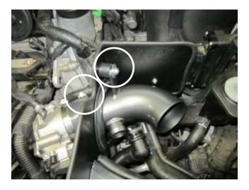
h) Install and tighten the washer and nut onto the mount (08160 & 444.460.04). Then make sure the AEM tube is fully seated in the hose on the throttle body and tighten the hose clamp.
