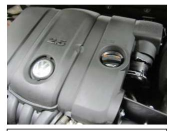
I) Re-install the engine cover onto the engine and push down to secure it.
