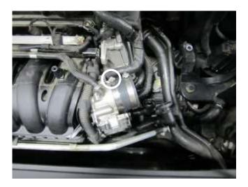
c) Install the hose and hose clamps onto the throttle body. Tighten the hose clamp closest to the throttle body at this time.
