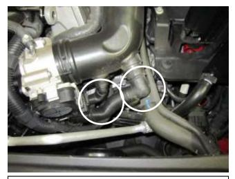
d) Detach both of the air injection connectors by squeezing the knurled area and pulling away from the stock intake tube. **Note: Some models have only one vent.**
