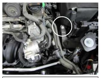
f) Remove the bolt shown. This bolt will not be reused.
