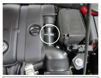
b) Release the pressure clamp at the engine cover outlet as shown and disconnect the stock intake hose from the engine cover.
