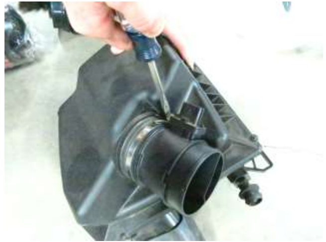
h. Loosen the clamp securing the MAF sensor housing to the factory air box and pull the housing out.
