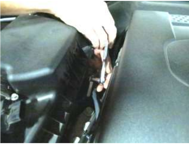
e. Remove the bolts securing the control module to the side of the factory air box. Keep these bolts.
