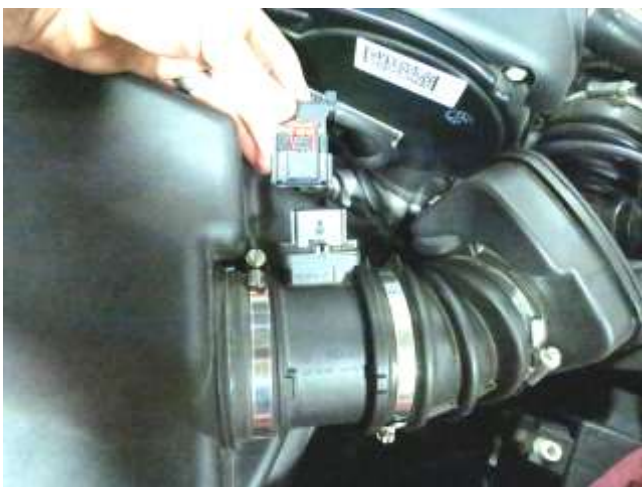
a. Disconnect wiring harness from the MAF sensor.
