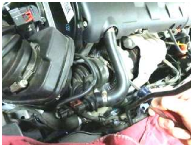
b. Loosen clamp securing the factory duct to the turbo-charger inlet.
