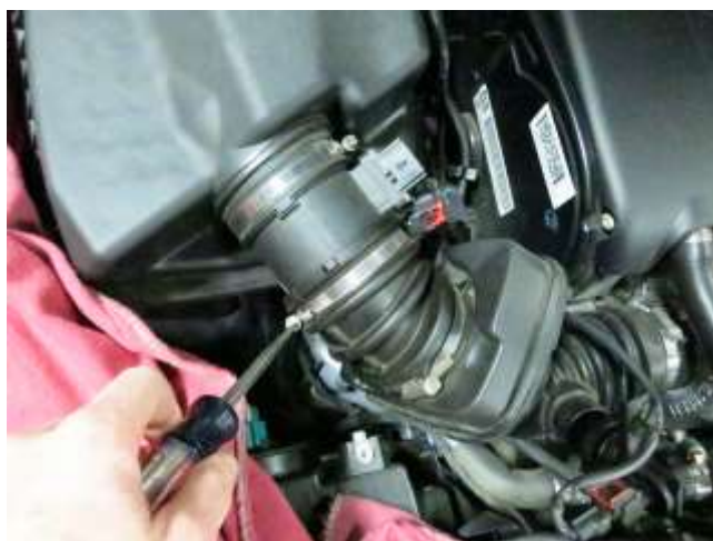
d. Loosen clamp retaining the factory duct to the MAF sensor housing and remove the duct.
