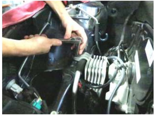
f. Lift the air box out and remove the nut on the motor mount shown above with a 15mm socket.
