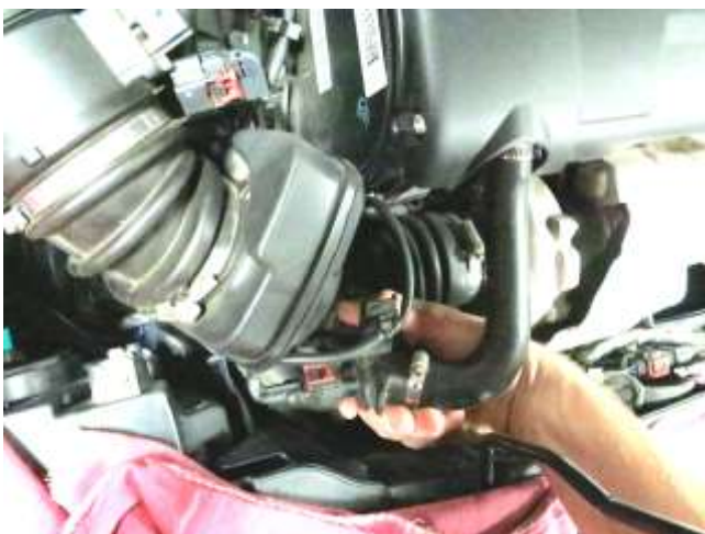
c. Disconnect crank vent tube by squeezing the retaining ring on the serrated flats and pulling free.
