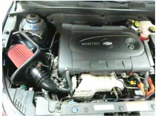
g. Finished installation of AEM Intake System.
