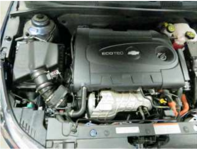
f. Factory air induction system.
