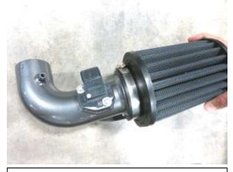
f. Install AEM filter(AEM-2127D) onto the intake tube with the hose clamp(AEM-9448) loosely fastened.
