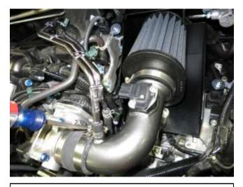
j. Adjust tube positon if needed and fasten the hose clamp on the coupler.
