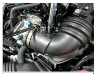
d. Loosen the hose clamp securing the intake tube to the throttle using a 8mm socket.
