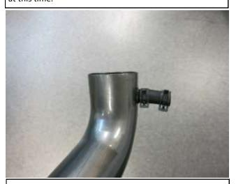
d. Install the provided hose and spring clamps onto the AEM intake tube. Trimming to 1.5" may be necessary.
