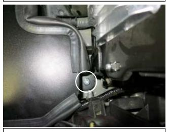
j. With the provided hardware, secure the AEM heat shield to the previously installed rubber mount on the frame rail.
