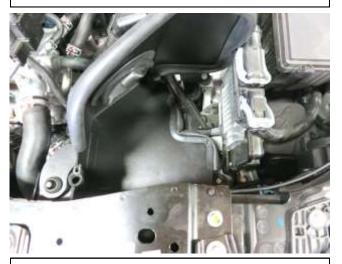
g. Install the AEM heat shield into the vehicle as shown, routing it around the electrical harness.
