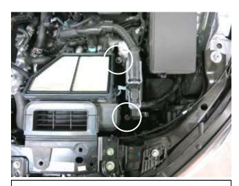
h. Remove the two bolts that secure the lower air box to the vehicle.
