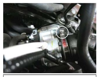
f. Loosen the hose clamp at the throttle body.
