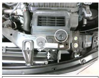
b. Remove the two push-in clips that secure the air box to the core support.
