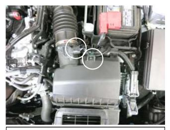
c. Depress the MAF (Mass Air Flow ) sensor connector tab and remove the connector from the sensor. Then, disconnect the green zip tie from the harness.
