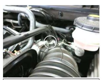
d. Squeeze the spring clamp on the vent line and remove the vent line from the stock intake tube.
