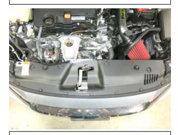
p. Re-install the front shroud cover on to the vehicle with the nine push-in clips removed in step 2a.
