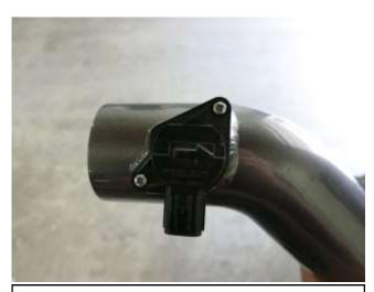
c. Install the MAF sensor into the AEM tube with the hardware that was removed in step 2l.
