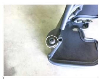
f. Install the grommet that was removed in step 2k. as shown.
