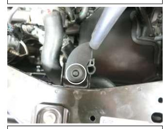
h. Seat the grommet onto the air box post as shown.
