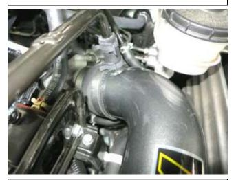
n. Connect the other end of the AEM intake tube into the coupler that was installed on the throttle body.
