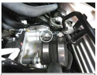
b. Install the provided coupler and hose clamps onto the throttle body. Tighten the circled hose clamp (30 in. lb.) at this time.
