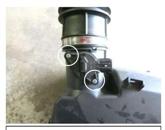
I. Remove the two screws and pull the MAF sensor from the stock upper air box. They will be reused in step 3c.
