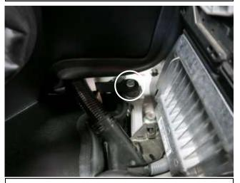
i. With the provided hardware, secure the AEM heat shield to the previously installed rubber mount towards the rear of the vehicle.
