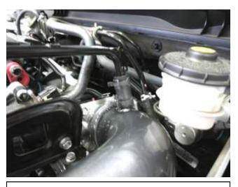
I. Align the previously installed hose on the AEM intake to the factory vent hard line and secure with the spring clamp.
