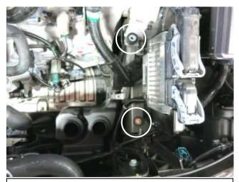
a. Install the two rubber mounts into the vehicle as shown.
