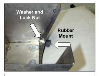
g. Install the supplied rubber mount onto the AEM<sup>®</sup> heat shield using one each of the supplied M6 washers and lock nuts.
