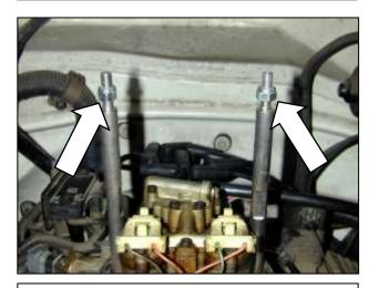
I. Thread two of the supplied 5/16-18 lock nuts on to the standoffs installed in step 3c. Leave approximately  $\frac{3}{4}$ " of thread exposed above the top of the nut. Place one 5/16" washer on top of each nut.
