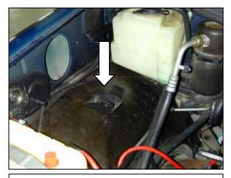
c. From inside the passenger side fender well, remove the two bolts holding the resonator hold down strap bracket. Remove the bracket.
