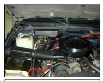
Factory air box system installed
