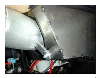
o. Install the AEM<sup>®</sup> inlet pipe into the coupler installed in the previous step. The bracket will line up with the rubber mount on the heat shield. Loosely secure the bracket with an M6 washer and lock nut. Refer to the following diagram for proper rubber mount installation.
