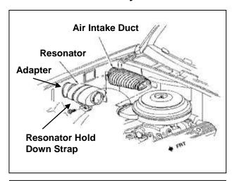
a. Remove the air intake duct, resonator, and adapter form the engine bay. The adapter is removed by gently squeezing the sides in to release the lip from the inner fender.
