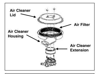
b. Remove the air cleaner housing and filter element by removing the two wing nuts. Remove the two mounting studs. Older models may be equipped with only one wing nut. On these models, remove the z-shaped rod from the center of the throttle body. Keep the air cleaner extension for use with the AEM® intake system.
