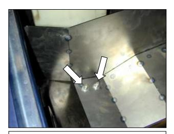
i. Align the hole in the heat shield with the heat shield bracket installed in step 3f. Secure using the supplied M6 bolt, fender washers and lock nut. Once the heat shield is in place, all three mounting bolts may be tightened.
