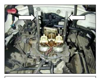
c. Thread the two hex-standoffs into the two rear throttle body mounting holes. Use one 5/16 washer under the hex portion of each standoff. The longer threaded end of the standoff is the end that threads into the intake manifold.
