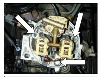
e. Remove the three bolts securing the throttle body to the intake manifold. Make note of the vacuum line connections at the front of the throttle body. Lift the throttle body and remove the old gasket.
