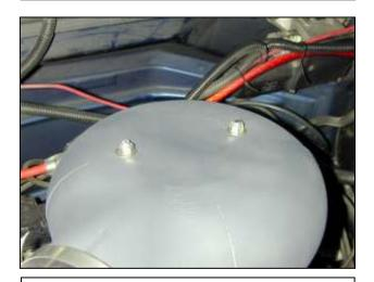
m. Install the air cleaner extension removed in step 2b. Reconnect the breather line on the back side. Test fit the AEM® intake plenum. The plenum should not rest on the washers installed in the previous step. Adjust the lock nuts until the top of the plenum compresses approximately ¼" for gasket sealing. Use the remaining washers and lock nuts to tighten down the plenum.
