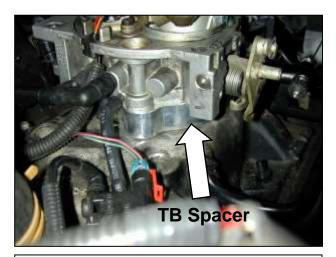
b. Place the AEM<sup>®</sup> throttle body spacer between the throttle body and intake manifold, using one of the supplied gaskets on each side.
