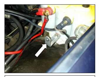
f. Remove the factory battery hold down bolt. Place the AEM<sup>®</sup> heat shield bracket under the head of the bolt and reinstall.
