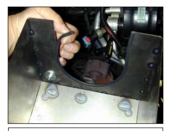
j. Install the rubber edge trim on to the heat shield where the intake pipe passes through.
