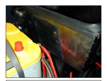
q. Apply the adhesive backed neoprene rubber to the heat shield directly opposite from the positive battery terminal.
