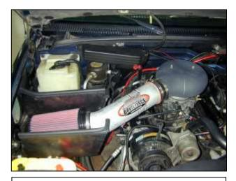
AEM® intake system installed
