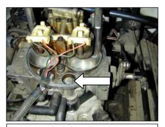
d. Place a 5/16 washer under the head of the supplied 5/16-18 bolt and install into the front throttle body mounting hole. Torque the hexstandoffs and bolt to 12 ft-lb.
