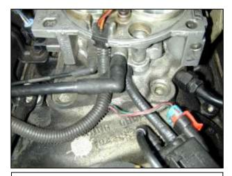
e. Reconnect any vacuum lines on the front of the throttle body that may have become dislodged. Secure the hard fuel line bracket removed in step 2d.
