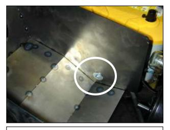
h. Loosely secure the heat shield in the engine bay using the supplied 5/16-18 bolts, washers and lock nuts. Insert the bolts up from the wheel well through the holes exposed in step 2c.
