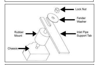
Proper installation of rubber mount assembly.
