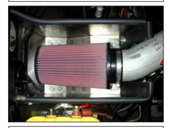
p. Install the AEM<sup>®</sup> air filter on to the end of the inlet pipe. Secure with the supplied hose clamp.
