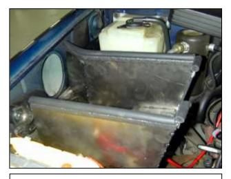
k. Install the foam rubber edge trim on to the top edge of the heat shield. Trim excess as necessary.
