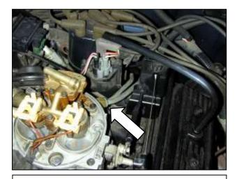
d. Follow the two fuel hard lines from the back of the throttle body down to the bracket on the transmission. Remove the nut securing the bracket to the transmission.
