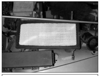
f. Remove the air filter element from the lower filter box.
