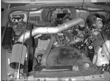
AEM® intake system installed
