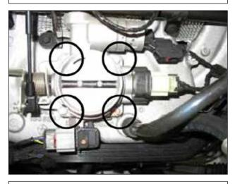
i. Remove the four bolts securing the throttle body to the intake manifold. After removal of the four bolts, place the throttle body spacer between the throttle body and the intake manifold. Install with the supplied gaskets and bolts, refer to the diagram on page 2 for the gasket placement.
