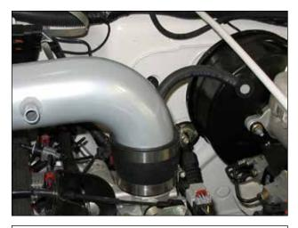
f. Insert the intake pipe into the rubber coupler attached to the throttle body.
