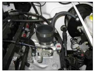
b. Secure the reducing coupler to the throttle body using the supplied #44 and #48 hose clamps.
