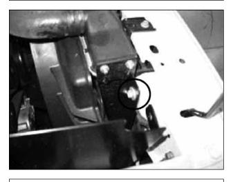
d. Remove the bolt securing the radiator to the core support. Slide the heat shield into position and re-insert the stock bolt through the heat shield hole and back through through the raditor support from which it was removed from.
