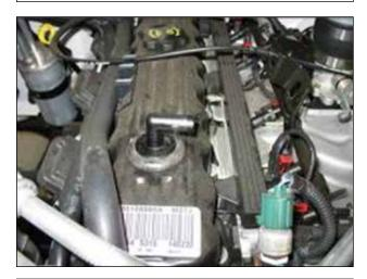
j. Twist the stock nipple carefully until it faces the driver side of the vehicle.
