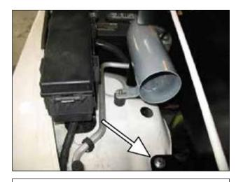
g. Align the intake pipe with the heat shield and rubber mount. After alignment is achieved, secure the heat shield with the supplied M8 bolt, washers and nut to the fender well of the vehicle.
