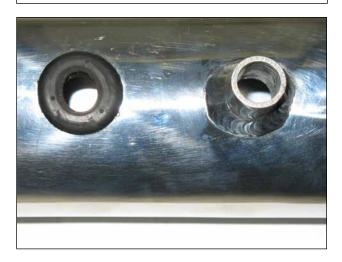
e. 2005-2006 Vehicles: Install the rubber grommet into the intake pipe as shown.
