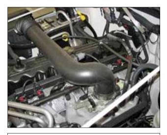
b. Loosen the hose clamp located at the throttle body.
