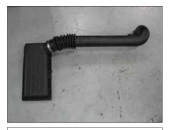
f. This is the intake tube and air filter lid after removal from the vehicle.
