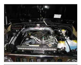
AEM® intake system installed
