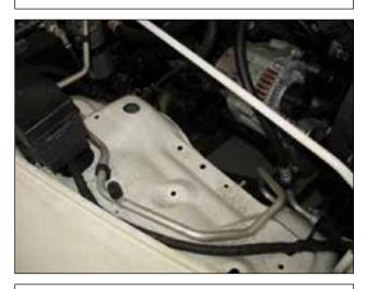
h. The factory air box housing removed.
