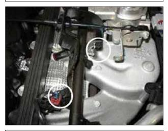
j. 2000-2006 Vehicles: Remove the 2 bolts on the throttle body linkage and replace with the supplied bolts and spacers.
