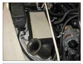
e. Remove the air filter lid from the air filter housing. Unclasp the four retaining clasps. Also be sure to disconnect the crank case breather hose from the lid.
