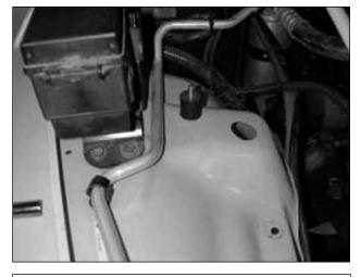
c. Install the supplied 6mm rubber mount. Use the supplied 6mm nut and 6mm washer. Attach the bolt and secure from underneath the fender well.
