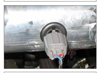
i. 2005-2006 Vehicles: Carefully install the IAT sensor into the intake pipe.1997-2004 Vehicles: Proceed to the next step.
