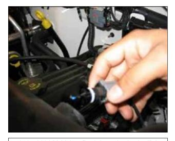
c. 2005-2006 Vehicles: Push in and twist the "Inlet Air Temperature" sensor out of the intake tube. 1997-2004 Vehicles: Proceed to the next step and disregard this step.
