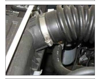
d. Loosen the hose clamp connecting the intake tube to the air filter lid.
