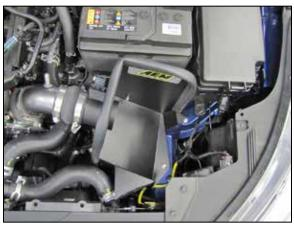
10. Install the heat shield and secure with the provided hardware. Install the AEM® intake tube into the couplers and adjust for best fit and secure with the provided hose clamps.
