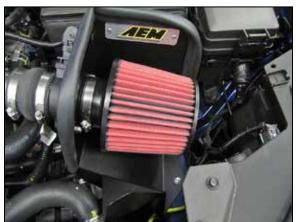
12. Install the AEM® air filter and secure with the provided hose clamp.
