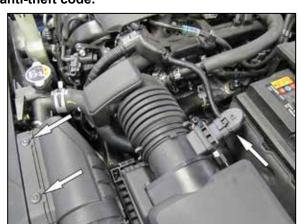
2. Disconnect the mass air sensor electrical connection. Disconnect the crank case vent line from the intake tube. Loosen the clamps at the throttle body and mass air sensor, then remove the factory intake tube. Push in the center of the pins that retain the fresh air intake duct and then remove the pins.
