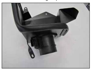
8. Remove the mass air sensor from the factory air filter housing and install it into the AEM® heat shield and secure with the provided hardware.
