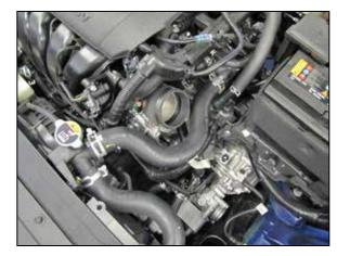
5. Install the provided hump coupler (08185) onto the throttle body and secure with the provided hose clamp.
