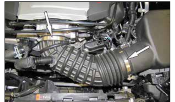
5. Loosen the hose clamps that secure the factory intake tube and then remove the intake tube from the vehicle.
