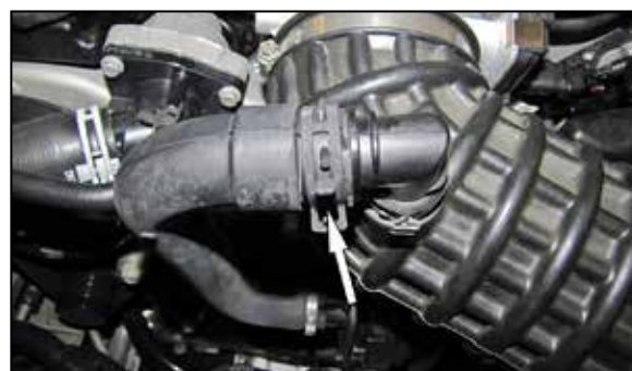
4. Release the spring clamp that secures the sound tube to the intake tube and then disconnect the sound tube.
