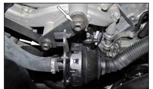
6. Remove the two bolts that secure the sound drum to the engine.
