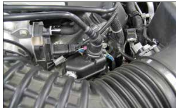
3. Disconnect the crank case vent quick disconnect from the factory intake tube.
