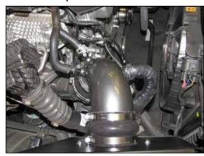
15. Install the AEM® intake tube into the couplers and adjust for best fit and secure with the provided hose clamps. Connect the vent lines and BOV hose and secure with the factory spring clamps.
