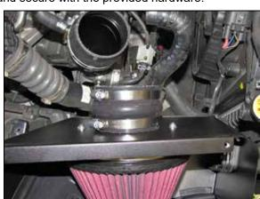
13. Install the provided hump coupler onto the filter adapter and secure with the hose clamp.
