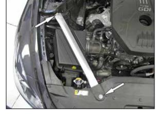
2. Remove the passenger side strut tower brace and set aside for later use.
