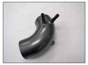
14. Install the vent fittings into the AEM® intake tube as shown.
