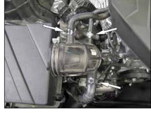
3. Release the spring clamps and disconnect the vent lines and BOV hose from the intake hose.
