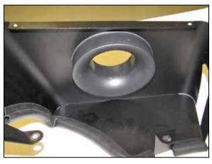
10. Install the radius filter adapter into the heat shield and secure with the provided hardware.
