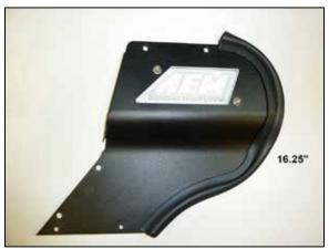
13. Install the AEM<sup>®</sup> logo into the heat shield and secure with the provided hardware. Install the edge trim onto the heat shield as shown.
