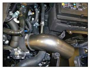
11. Install the AEM<sup>®</sup> intake tube into the coupler and connect the crank case vent hose and secure with the factory clamp.
