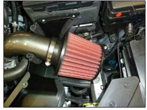
12. Install the AEM<sup>®</sup> air filter and secure with the provided hose clamp.
