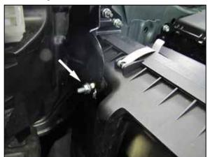
9. Remove the nut that secures the air filter housing to the bracket attached to the fender.
