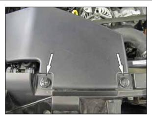
3. Remove the two clips that secure the fresh air intake duct.
