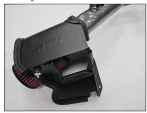
18. Install the AEM® intake tube trough the heat shield and install the AEM® air filter onto the tube and secure with the provided hose clamp.
