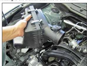
10. Remove the complete air filter housing assembly from the vehicle.
