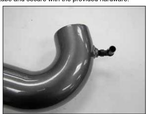
16. Install the 90° vent fitting into the AEM® intake tube as shown.
