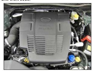
2. Lift up the decorative engine cover and remove it from the engine.
