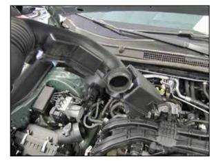
7. Remove the factory intake tube from vehicle.
