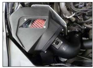
14. Install the assembly into the vehicle so the intake tube engages the coupler and the mounting studs engage the mounting grommets. Tighten hose clamp.
