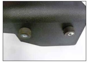
7. Install the two rubber mounted studs onto the AEM air filter housing using the provided hardware.
