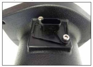
10. Remove the sensor from the factory intake tube. Install the sensor into the intake tube using the provided hardware.
