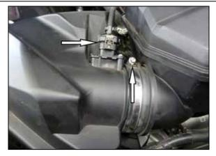
2. Disconnect the temperature sensor electrical connection. Loosen the hose clamp connecting the intake tube to the factory air filter housing, separate the tube from the housing. Lift the air filter housing up and remove it from the vehicle.
