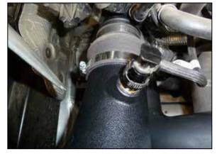
15. Connect the CCV hose to the fitting installed into the intake tube.
