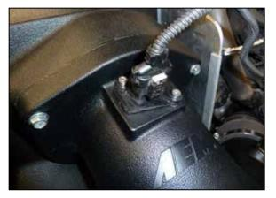
16. Reconnect the sensor electrical connection.
