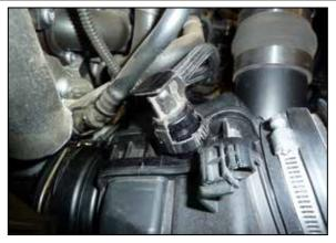
3. Pinch the locking tab s on the CCV hose connection and then disconnect the CCV hose from the factory intake tube.
