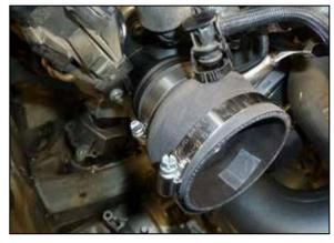
13. Install the provided coupler onto the turbo inlet.
