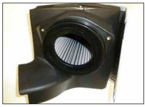
11. Place the air filter into the AEM air filter housing.
