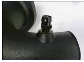
9. Install the provided CCV fitting into the AEM intake tube. Be sure to apply thread sealer before installing the fitting into the intake tube.
