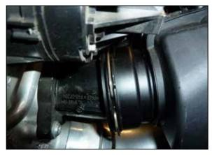
4. Remove the clip the locks the intake tube to the turbo inlet and then disconnect the tube from the turbo and remove it from the vehicle.
