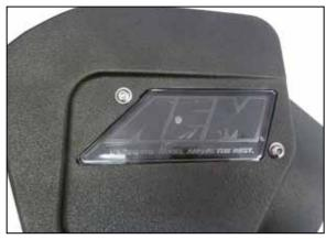
6. Install the AEM window into the air filter housing using the provided hardware.
