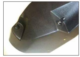
5. Install the provided mounting studs onto the AEM air filter housing using the provided hardware.
