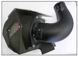
12. Install the AEM tube onto the filter housing and secure with the provided hardware.
