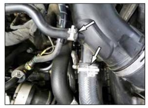
4. Release the spring clamps that secure the BOV hose and vent line, then disconnect the lines rom the factory intake tube.
