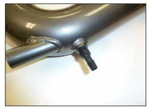
14. Install the provided vent fitting into the K&N intake tube as shown.
