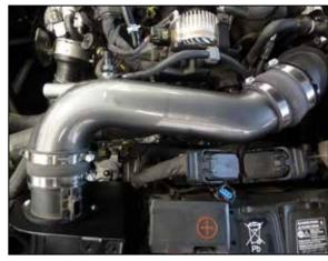
15. Install the intake tube into the hump coupler and then into the straight coupler, adjust for best fit and then secure with the provided hose clamps.
