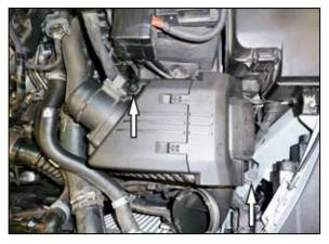
6. Remove the two bolts that secures the air filter housing and then remove the filter housing from the vehicle.
