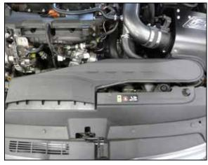
21. Reinstall the Fresh air intake duct.
