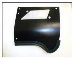
19. Install the AEM window into the heat shield lid with the spacer between the window and the lid. Secure the assembly with the provided hardware. Install the 11.5 section of edge trim onto the lid as shown.
