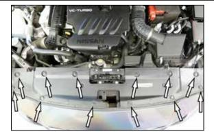
2. Remove the twelve retaining pins that secure the radiator valence. Then remove the valence from the vehicle.
