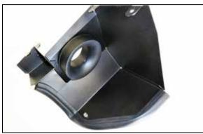
12. Cut a section of edge trim to 18" and install it onto the heat shield as shown.
