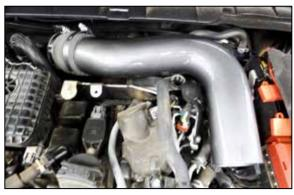
17. Install the rear intake tube into the coupler but do not tighten the hose clamp at this time.
