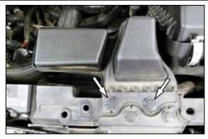
3. Remove the two retaining pins that secure the fresh air duct to the core support.
