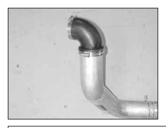
f. Attach the 3" side of the silicon elbow to the inlet pipe. Secure elbow to the inlet pipe. The open end connects to the turbo inlet which sits horizontal.
