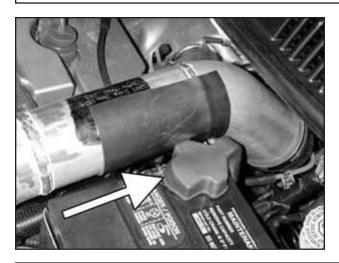
i. Make sure neoprene rubber adhesive clears the positive battery terminal. Make sure the (+) post protector on the battery is not damaged, cracked or melted. If any of the conditions exist, you must replace before completing the installation of the AEM® intake system. Failure to not follow these instructions will void warranty.
