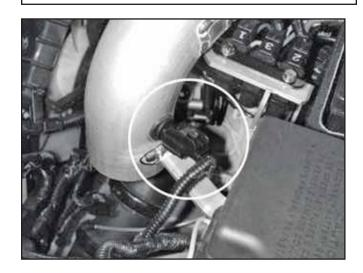
I. Reinsert IAT sensor into the rubber grommet.
