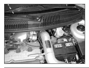
g. Attach the other end of the silicon coupler to the turbo inlet. Line up the bracket on the inlet pipe to the rubber mount. Secure the hose clamp.
