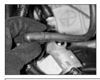
o. Insert vacuum fitting into the vacuum cap left from the installation Step 2d.
